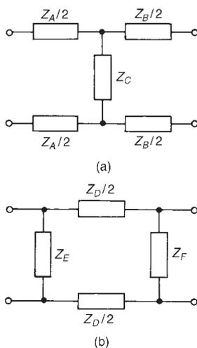
**Figure 41.2** (a) *Balanced T-network*, (b) *Balanced  $\pi$ -network*
