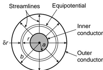
Figure 40.11 Electric field between two concentric cylinders
