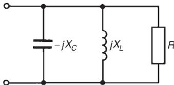
**Figure 29.1** Parallel  $R$ - $L$ - $C$  circuit
