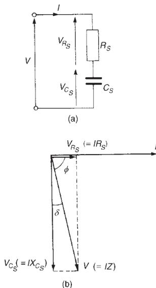
**Figure 39.2** (a) Circuit diagram (b) Phasor diagram
