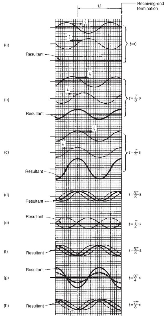
**Figure 44.10** Current waveforms on an open-circuited transmission line
