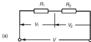
$$V_1 = \left( \frac{R_1}{R_1 + R_2} \right) V$$
