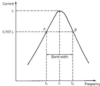
**Figure 28.6** Bandwidth and half-power points  $f_1$  and  $f_2$
