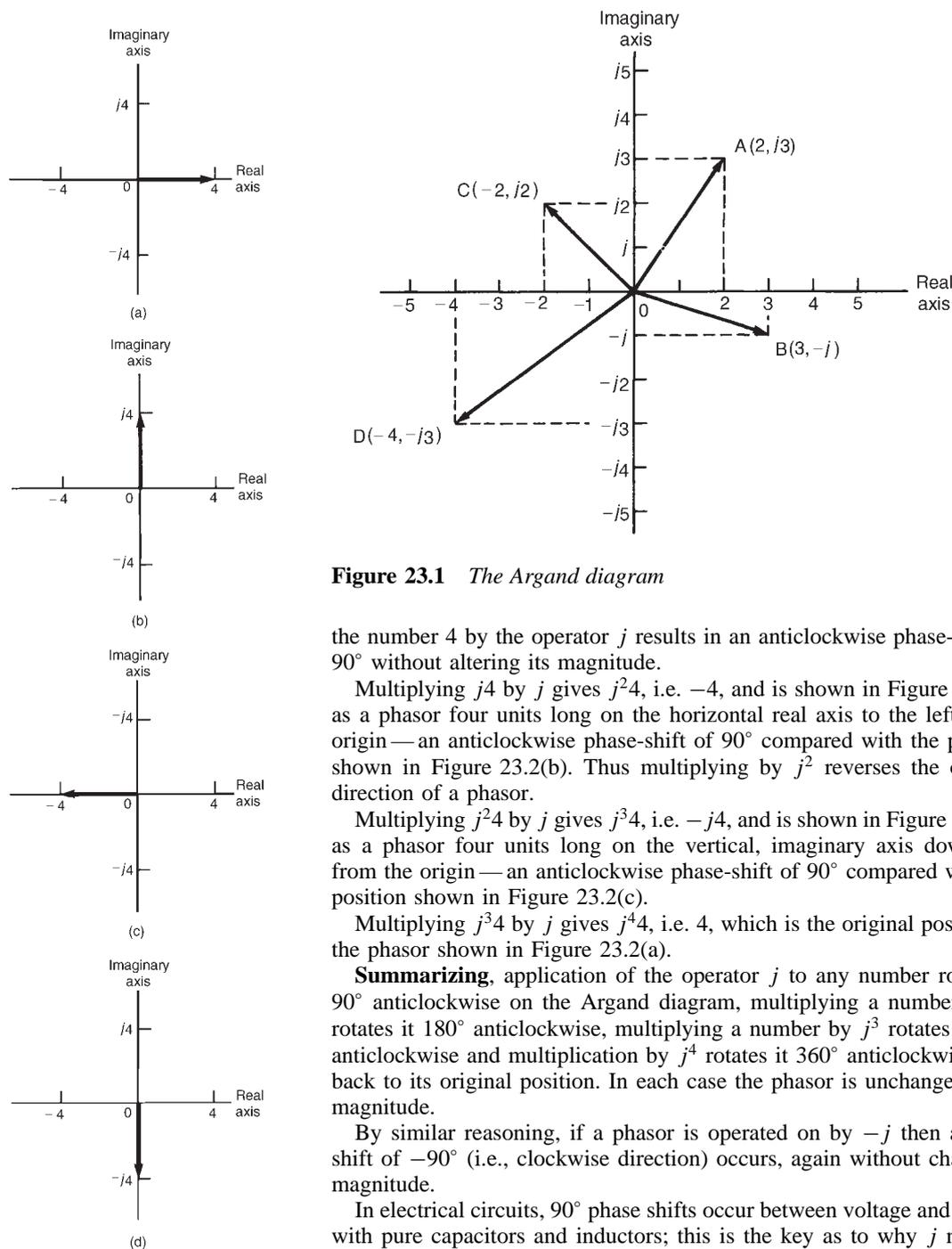
**Figure 23.1** *The Argand diagram*
