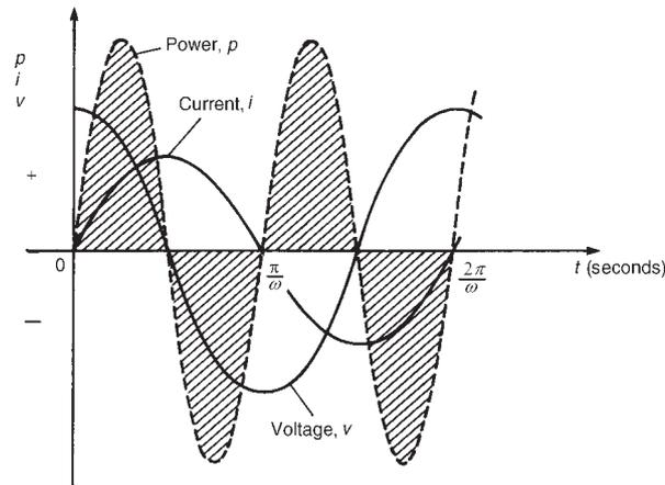
**Figure 26.2** Power in a purely inductive a.c. circuit
