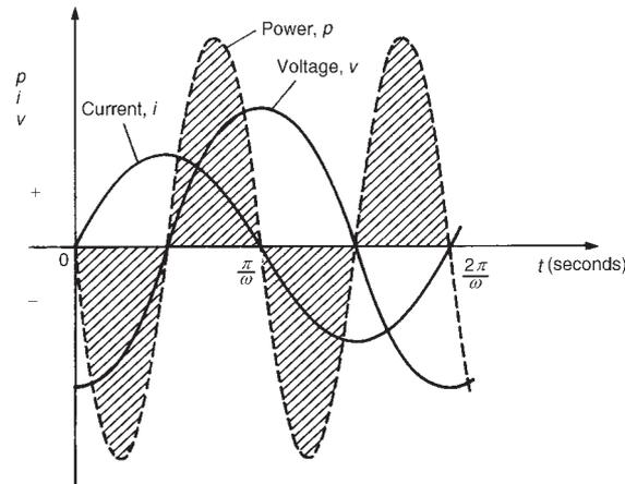
**Figure 26.3** Power in a purely capacitive a.c. circuit
