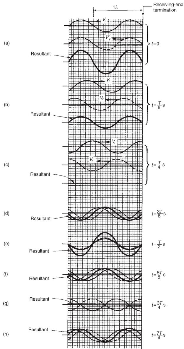
**Figure 44.12** Voltage waveforms on an open-circuited transmission line
