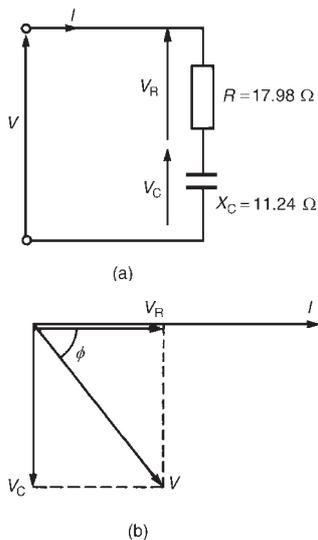
**Figure 25.2** (a) Circuit diagram, (b) Phasor diagram
