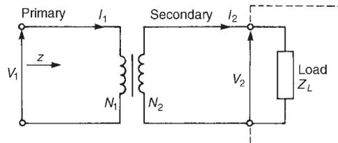
Figure 35.11 Matching impedance by means of a transformer
