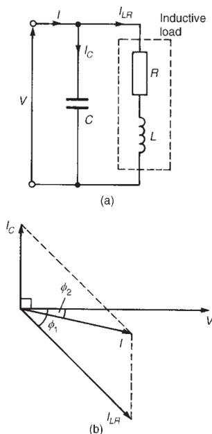
**Figure 26.11** (a) Circuit diagram (b) Phasor diagram
