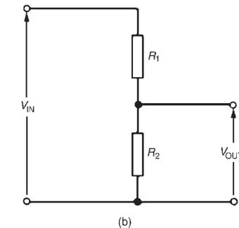
The circuit shown in Figure 5.5(b) is often referred to as a **potential divider** circuit. Such a circuit can consist of a number of similar elements in series connected across a voltage source, voltages being taken from connections between the elements. Frequently the divider consists of two resistors as shown in Figure 5.5(b), where
