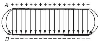
Figure 6.1 *Electrostatic field*
