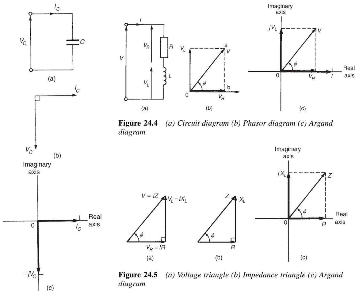
**Figure 24.4** (a) Circuit diagram (b) Phasor diagram (c) Argand diagram
