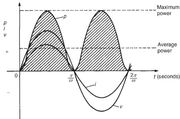
**Figure 26.1** *The waveforms of  $v$ ,  $i$  and  $p$*
