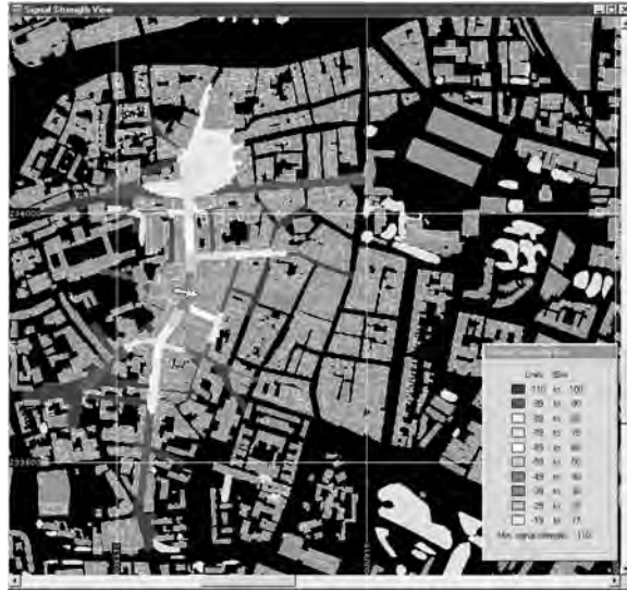
FIGURE 74.4 NP WorkPlace coverage plot of a city street microcell. The map gridsize is 500 meters.
