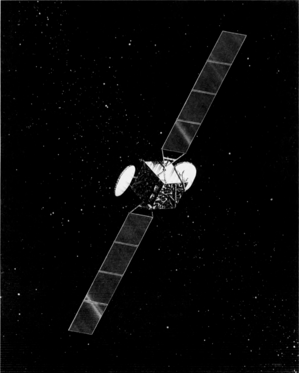
FIGURE 56.7 Galaxy VII, launched in 1993, is a medium-power Hughes HS-601 satellite that provides 24 low-power C-band and 24 medium-power Ku-band transponders to the U.S. market. It is used by cable TV and over-the-air broadcasting networks to distributed programming to affiliates. (Photograph courtesy of Hughes Space and Communications Company.)
