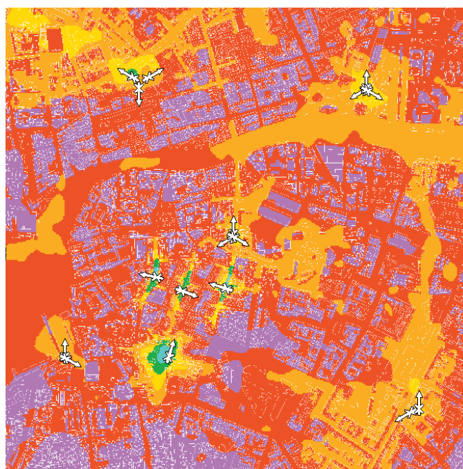
FIGURE 74.12 The required transmit power for MSs using the speech service, when the level of offered traffic has been increased by a factor of four.
