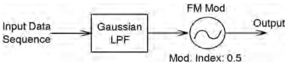
FIGURE 24.13 Generation of GMSK signal; LPF is low-pass filter.
