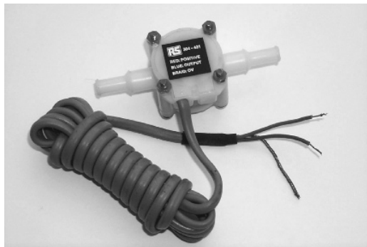
FIGURE 21.9: Liquid flow sensor (digital output)
