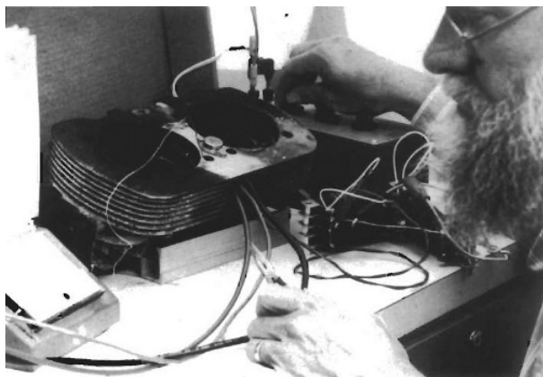
FIGURE 6.4: When using high-power amplifiers, there are there are certain problems you just never have if you use a big-enough heat sink. This heat sink’s thermal resistance is lower than 0.5°C/W. (Photo copyright Peggi Willis.)
