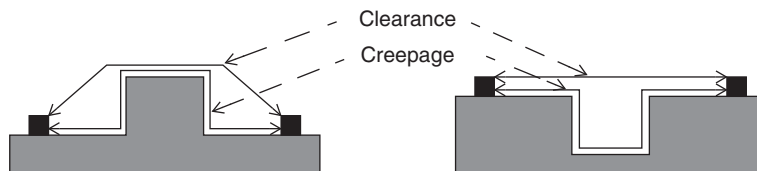
FIGURE 39.2: Creepage and clearance distance
