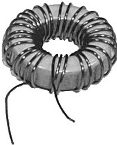
FIGURE 1.55: A practical coil contains inductance and resistance
