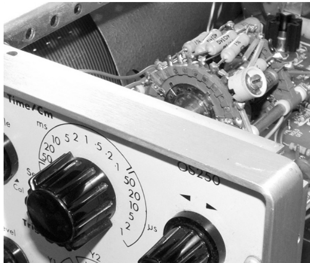
FIGURE 1.94: C-R circuits are widely used in electronics. In this oscilloscope, for example, a rotary switch is used to select different C-R combinations in order to provide the various timebase ranges (adjustable from 500 ms/cm to 1 \mu\text{s/cm} ). Each C-R time constant corresponds to a different timebase range.
