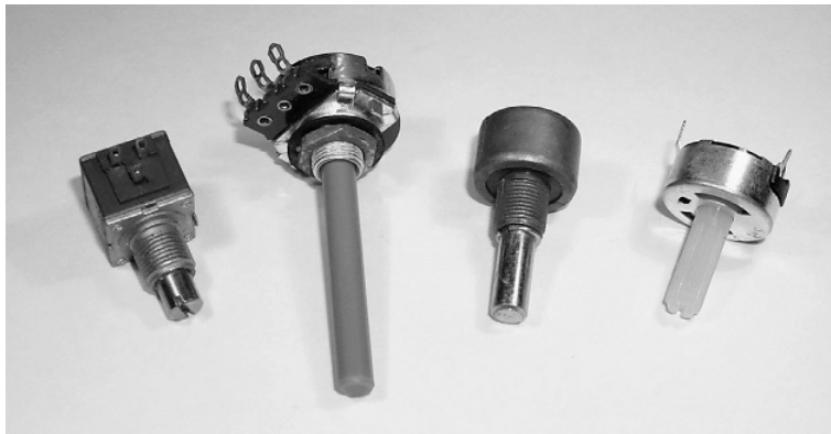
FIGURE 1.40: A selection of common types of carbon and wirewound variable resistors/potentiometers
