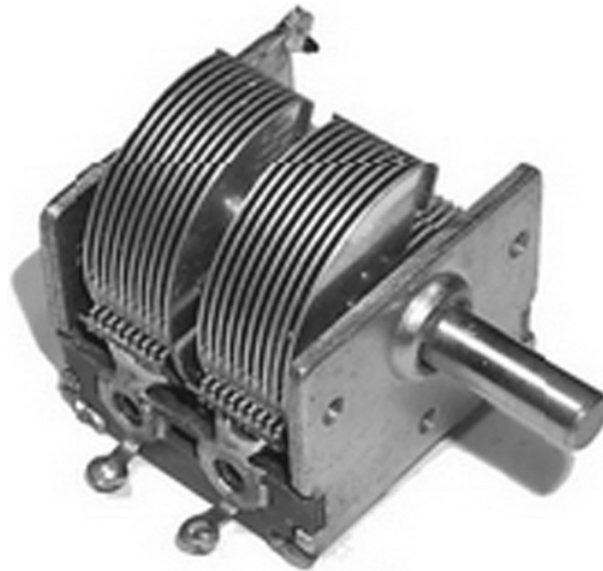
FIGURE 1.54: An air-spaced variable capacitor. This component (used for tuning an AM radio) has two separate variable capacitors (each of 500 pF maximum) operated from a common control shaft.
