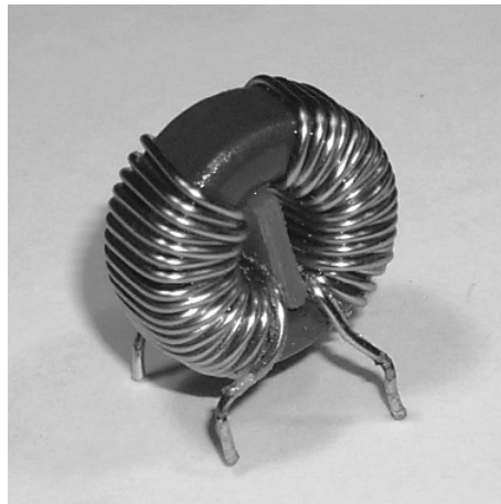
FIGURE 1.127: This small 1:1 ratio toroidal transformer forms part of a noise filter connected in the input circuit of a switched mode power supply. The transformer is wound on a ferrite core and acts as a choke, reducing the high-frequency noise that would otherwise be radiated from the mains supply wiring
