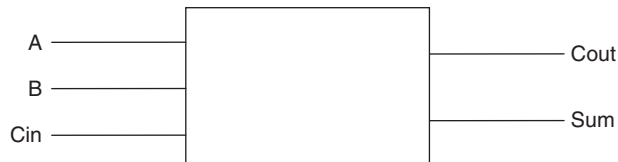
FIGURE 10.9: One-bit full-adder cell
