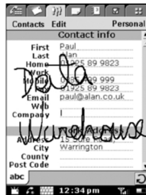
FIGURE 42.40 Write-anywhere text input method for mobile devices. Example of an Address Book application with the Company field appearing with focus. Hand written input is not restricted to a delimited area of the screen but rather can occur anywhere. The company name “Data Warehouse” has been written.
