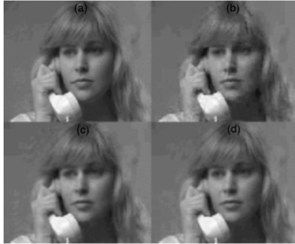
FIGURE 42.29 150th Frame of original: (a) “Suzie” sequence and its compressed version at 64 kbit/s using, (b) H.261, (c) baseline H.263, and (d) Full-option H.263.
