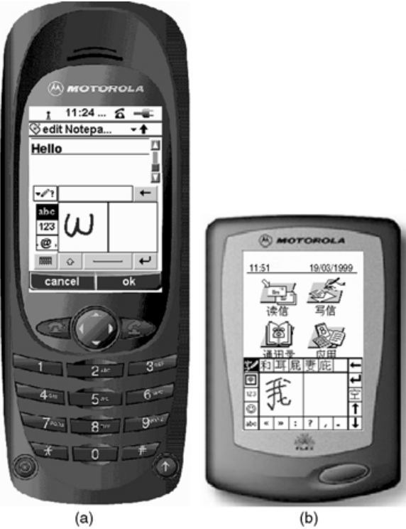
FIGURE 42.37 Character-based text input method on today’s mobile devices. In (a), user interface for English character input on a cellular phone. In (b), user interface for Chinese character input on a 2-way pager.
