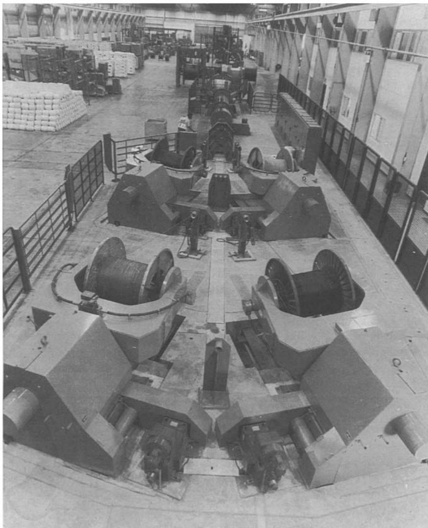
**Fig. 25.7** Drum-twister laying-up machine
