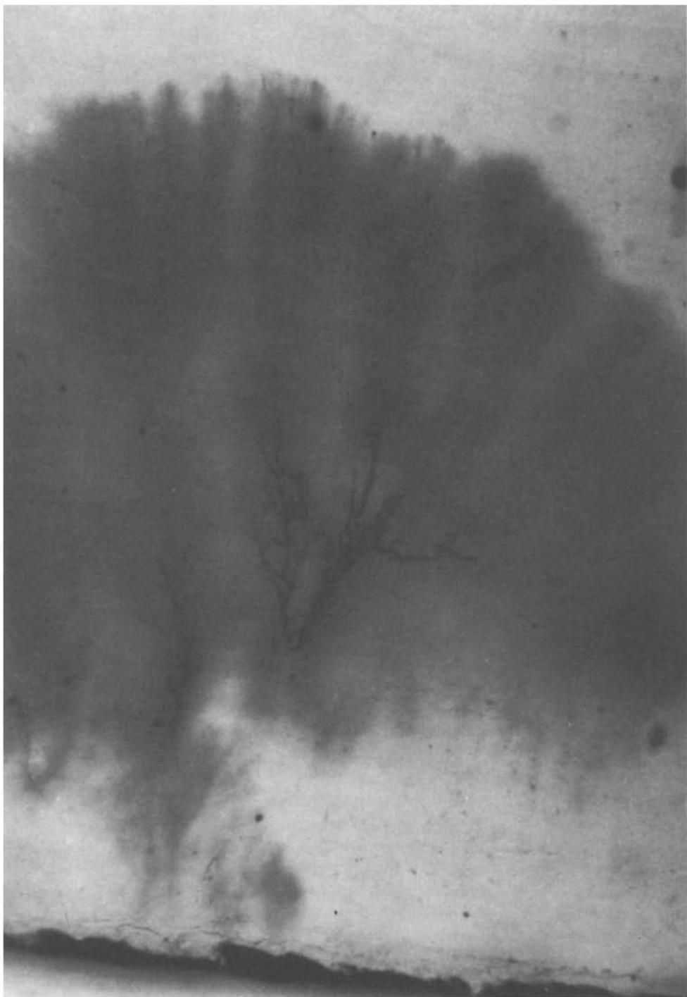
**Fig. 24.4** Electrical tree forming within a water tree
