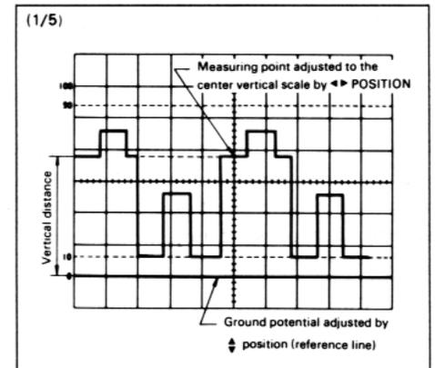
Fig. 22. Instantaneous DC voltage measurement.
