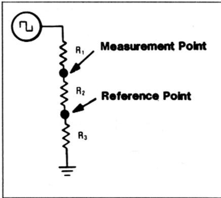
**Fig. 24. Voltage measurement with reference other than earth ground.**
