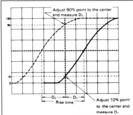
**Fig. 32. Alternative rise time and fall time measurement**
