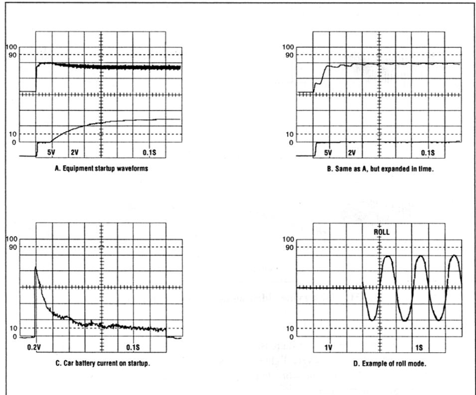
**Fig. 48. DSO stored waveforms.**
