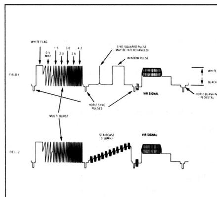
**Fig. 46. Typical VITS signal**
