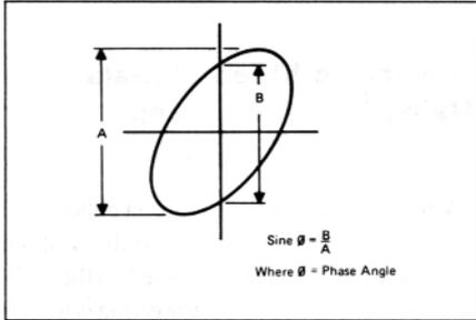
**Fig. 41. Phase measurement, X-Y operation.**
