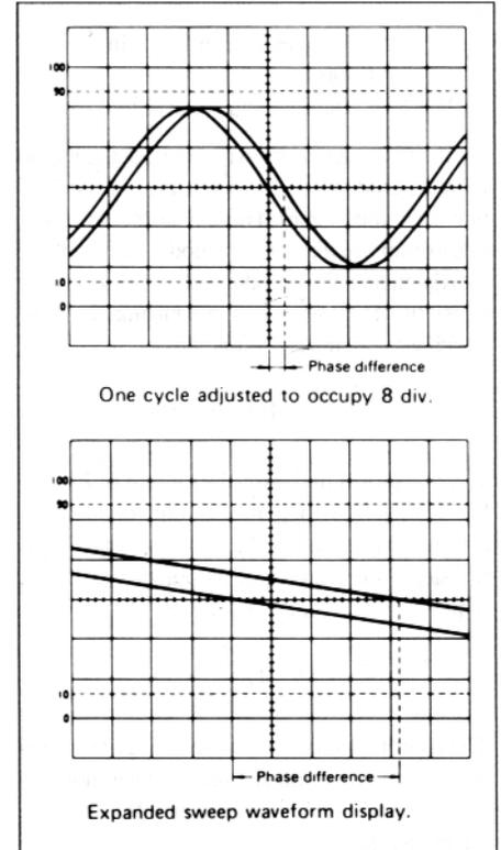
**Fig. 36. Measuring small phase difference.**
