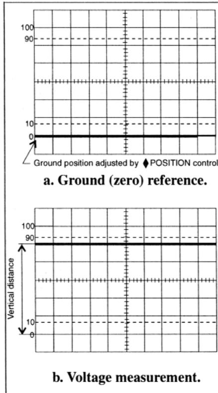
Fig. 21. DC voltage measurement.
