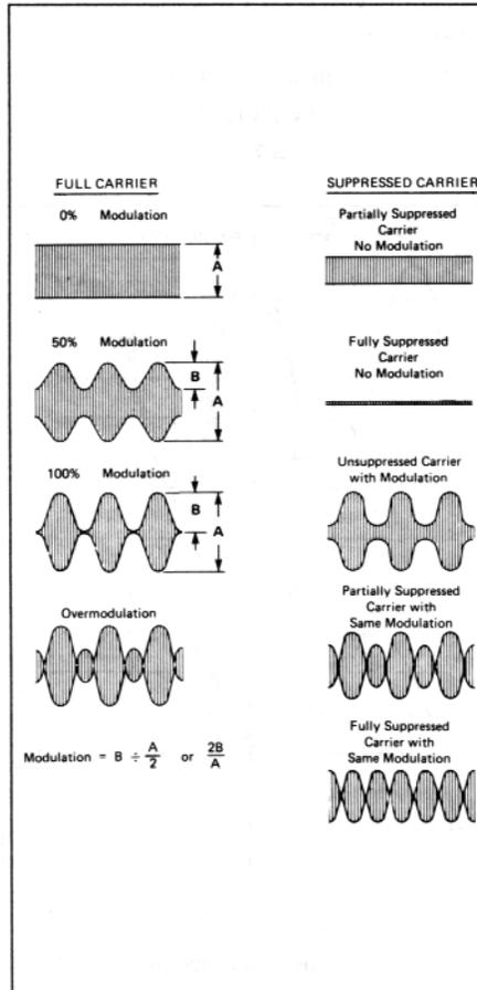
**Fig. 33. Percent of modulation measurement**
