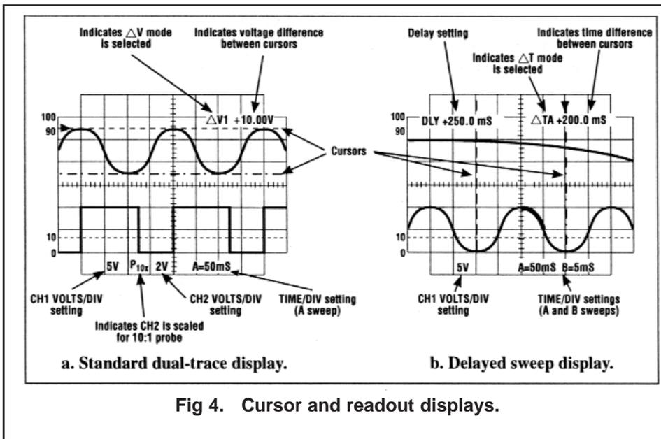
**Fig 4. Cursor and readout displays.**
