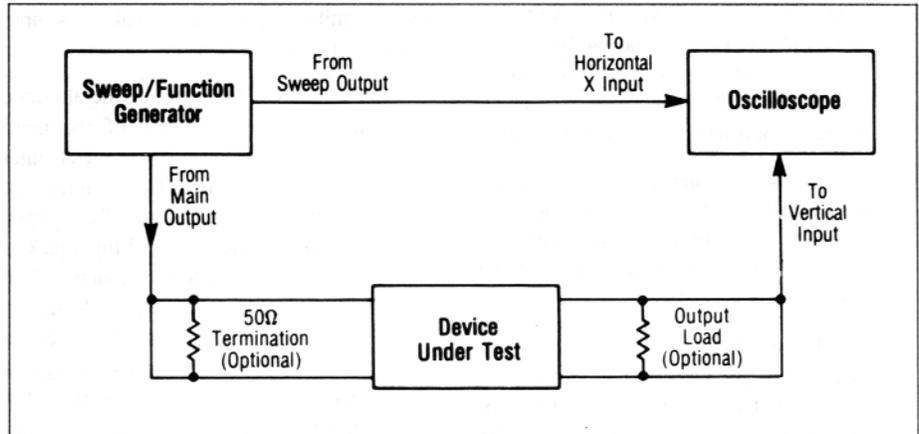
**Fig. 43. Frequency response test set-up.**
