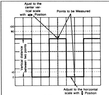
**Fig. 25. Differential voltage measurement.**
