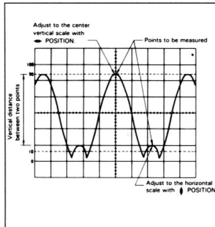
**Fig. 23. Voltage measurement.**
