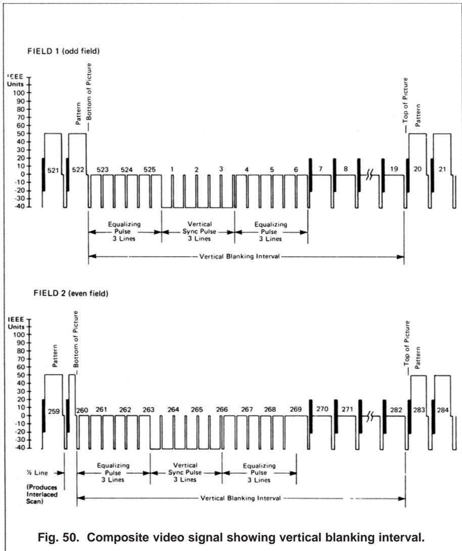
**Fig. 50. Composite video signal showing vertical blanking interval.**
