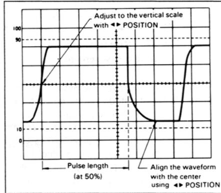
**Fig. 30. Pulse width measurement.**
