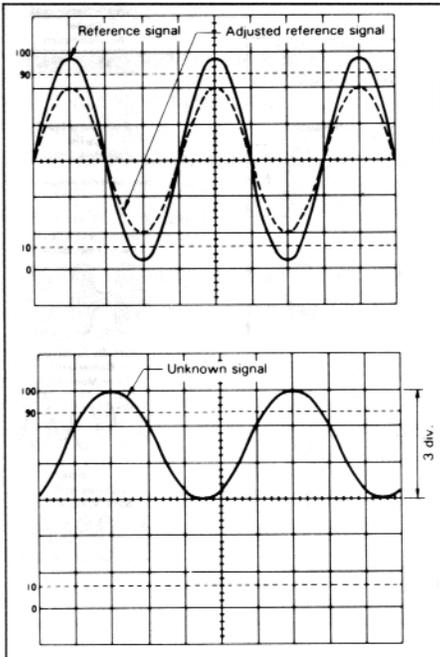
**Fig. 37. Voltage measurement, relative, method**
