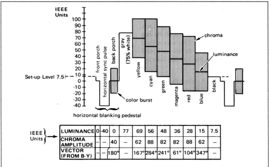
**Fig. 49. One horizontal line of NTSC color bars signal.**
