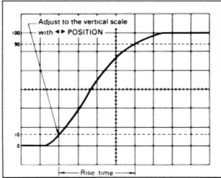
**Fig. 31. Rise time and fall time measurement**
