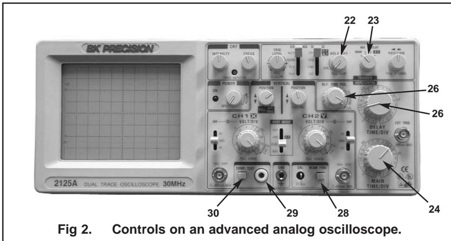
**Fig 2. Controls on an advanced analog oscilloscope.**
