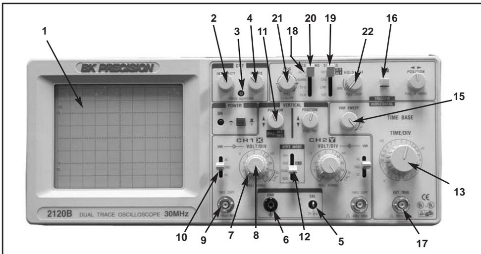
**Fig 1. Basic controls and indicators.**
