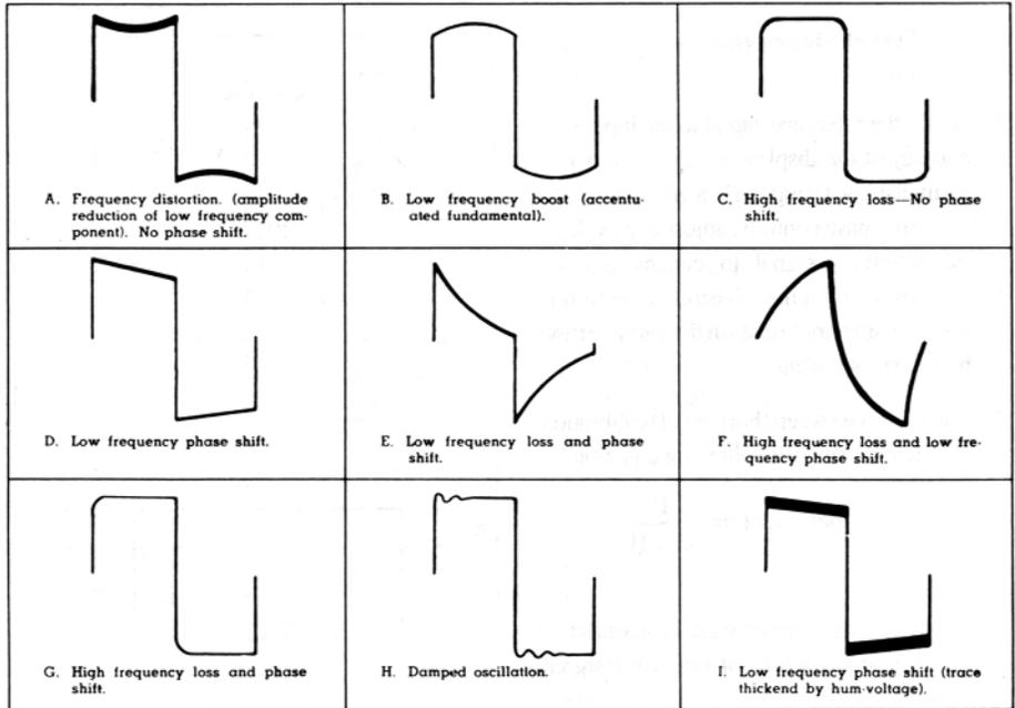
**Fig. 39. Square wave analysis waveform.**
