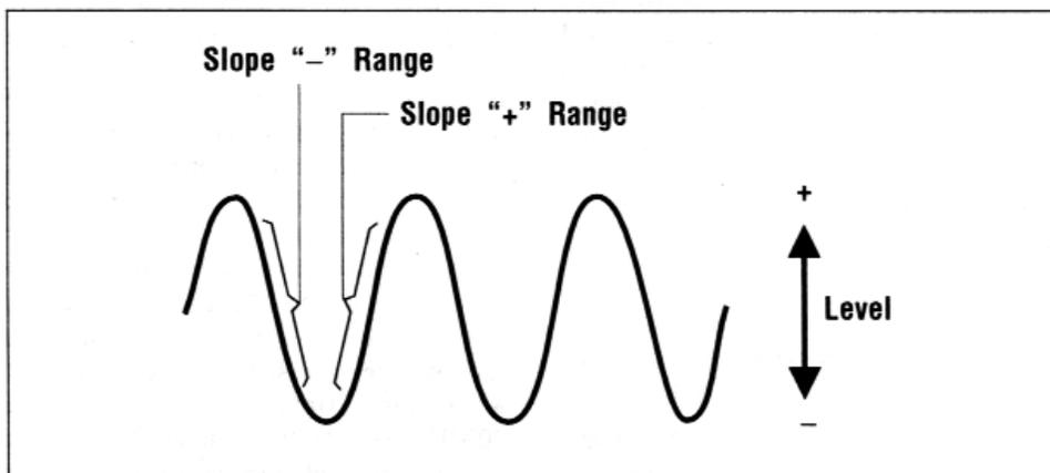
Fig. 6 Function of SLOPE and LEVEL controls
