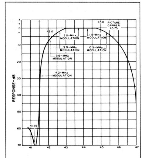
**Fig. 47. Color TV IF amplifier response curve**
