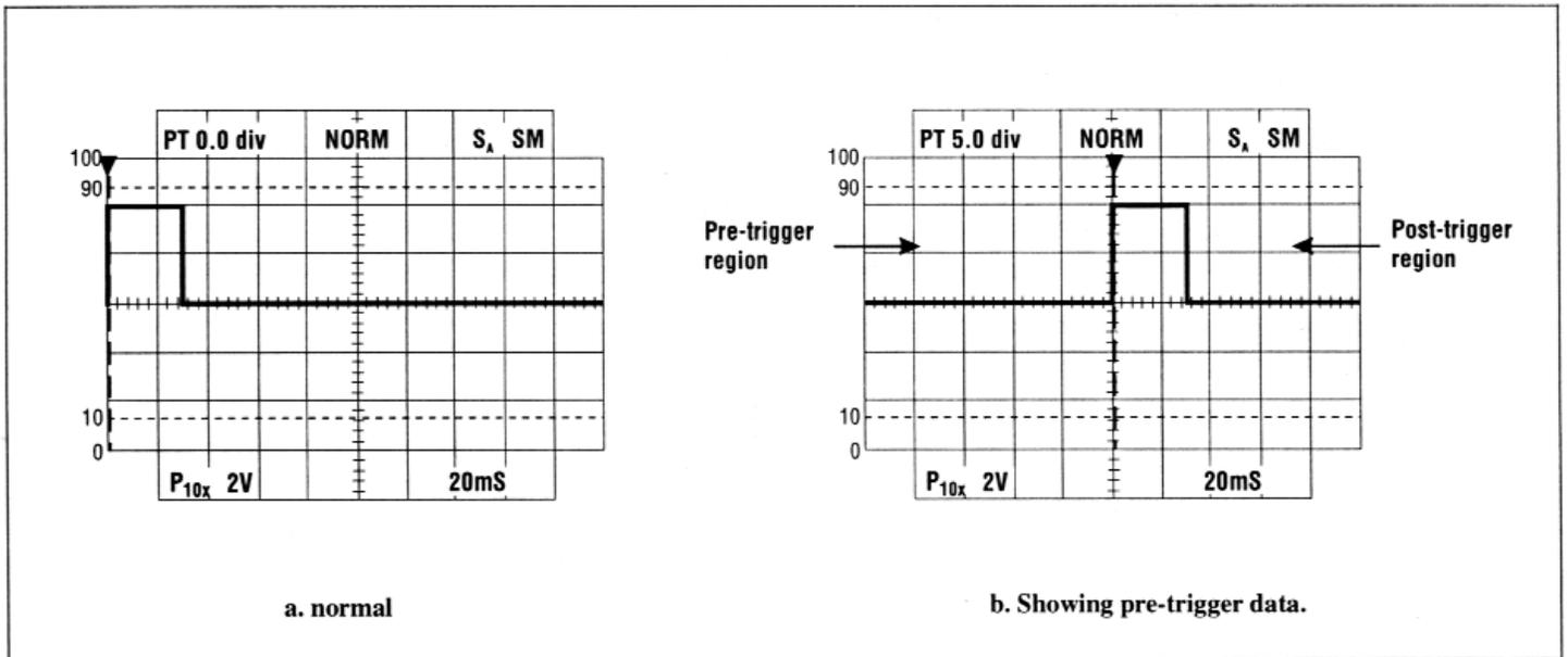
**Fig. 10 Capture of a cone-time event.**
