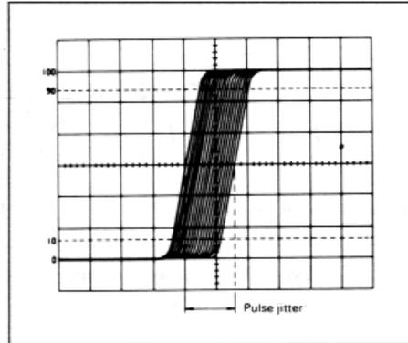
**Fig. 44. Pulse jitter measurement**
