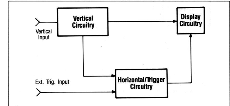
Fig. 11. Simplified oscilloscope block diagram.
