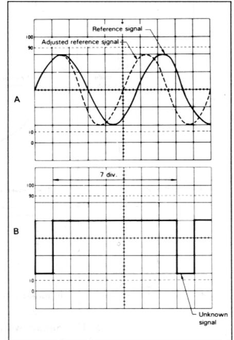
**Fig. 38. Period measurement, relative, method**
