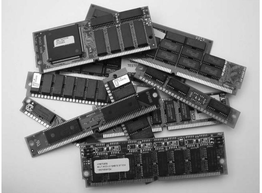
**Photo 1.9** *Various PC memory devices with capacities varying from 1 to 256 MB*
