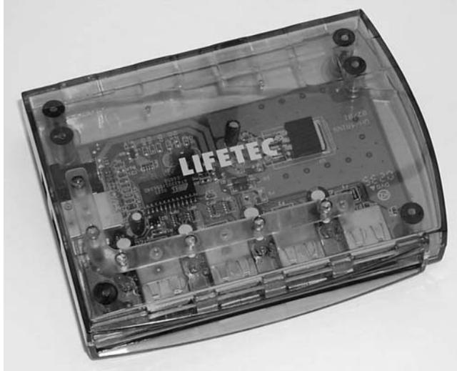
**Photo 2.15** *A low-cost USB four-port hub*
