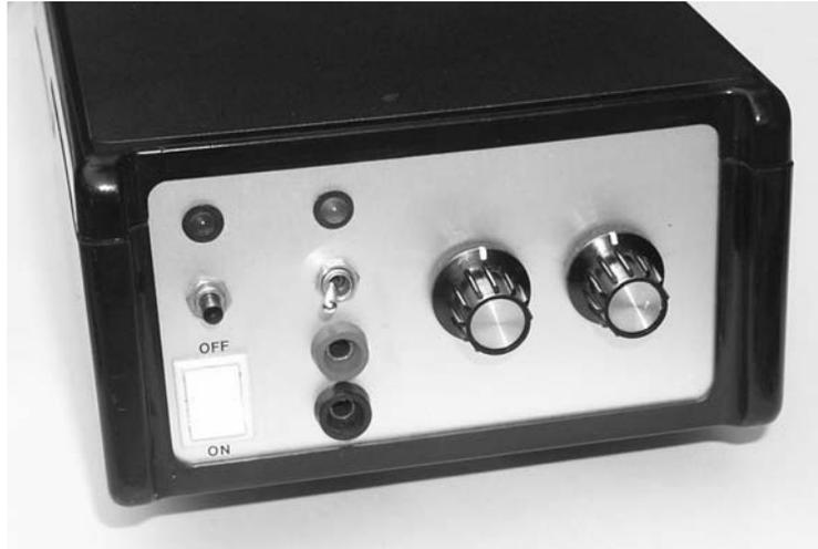
**Photo 11.4** *The prototype sound card oscilloscope interface*
