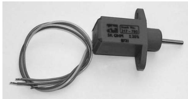
**Photo 9.2** *Linear position sensor (analogue output)*
