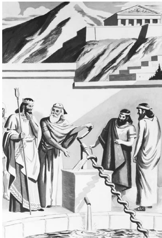
The Archimedean screw lifted water from one level to another. (Bettmann/Corbis. Reproduced with permission.)
