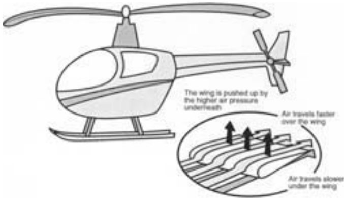
Figure 7.2. The lift of a helicopter.
