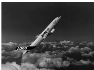
Figure 3.1. An Airbus research aircraft about to go into free fall, which it can sustain for up to 22 s. Image courtesy Novespace/Airbus.
