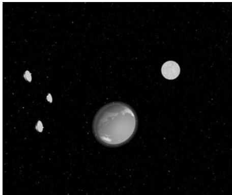
Figure 22.9. An artist's view of how LISA would look in orbit around the Sun, about 20^\circ behind the Earth. The three spacecraft follow free orbits around the Sun, chosen so that they remain in formation, always facing the Sun and lying in a plane tilted at 60^\circ to their orbits. The sizes of the spacecraft, Sun, and Earth are, of course, not drawn to scale. Image by Chris Osland and Jonathon Copeland, Rutherford Appleton Laboratory, used with permission.
