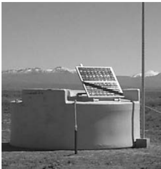
Figure 27.3. One detector of the Pierre Auger Observatory, an array of 1600 similar units being constructed in Argentina, able to observe high-energy cosmic rays striking anywhere in an area of 3000 km 2 . It is hoped that this will provide enough data to solve the mystery of the ultrahigh-energy cosmic rays. Image courtesy Pierre Auger Observatory.
