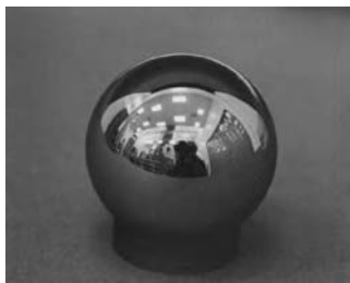
Figure 19.5. This fused-quartz sphere coated with superconducting niobium is one of the gyroscopes carried on GP-B. The size of a table-tennis ball, it is so spherical that its irregularities are nowhere more than 40 atoms high. This is just one of many challenges that have been met in designing this extraordinarily sensitive satellite. Image courtesy of Gravity Probe B.
