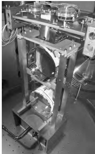
Figure 22.8. One of the mirror assemblies for the GEO600 detector. The bottom piece is the mirror, the upper disk a balancing part of the suspension. The mirrors are made of high-quality fused silica (quartz) and are suspended from fibers made of the same material. The quality of the suspension is such that if the mirror pendulum were set swinging and left alone in the vacuum system, it would swing for many months before the amplitude reduced by half. Image courtesy of GEO600.
