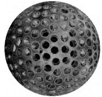
Figure 19.6. The LAGEOS satellite is the complete opposite of GP-B. It is a passive satellite, with no working components. Covered in mirrors, its only job is to reflect laser beams back to Earth, which are used in range-finding to find its exact position. The relativity experiment is a spin-off from the satellite's main mission, which is to track continental drift by measuring the motion of the ground stations that track the satellites. From the tracking data, however, scientists are beginning to discern the gradual precession of the orbit of one of them induced by the Lense-Thirring effect. Image courtesy GSEC.
