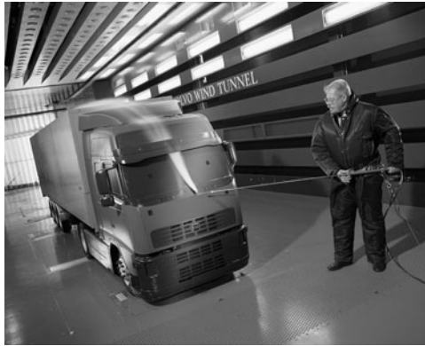
Figure 14.1 Aerodynamic testing of a truck with smoke in a wind tunnel.
