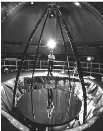
Figure 5.20 Parabolic liquid mercury mirror formed of the surface of the rotating vessel.
