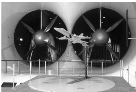
Figure 1.4 Model of F-18E in a 30 ft \times 60 ft wind tunnel at the NASA Langley Research Center.
