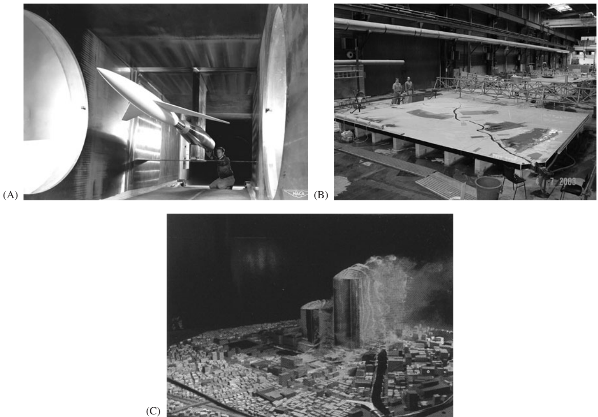
Figure 9.1 (A) Model of an aircraft in a wind tunnel. (B) scale model of a section of the Mississippi River. (C) Model of San Antonio, Texas, used for determining wind patterns in this urban environment.
