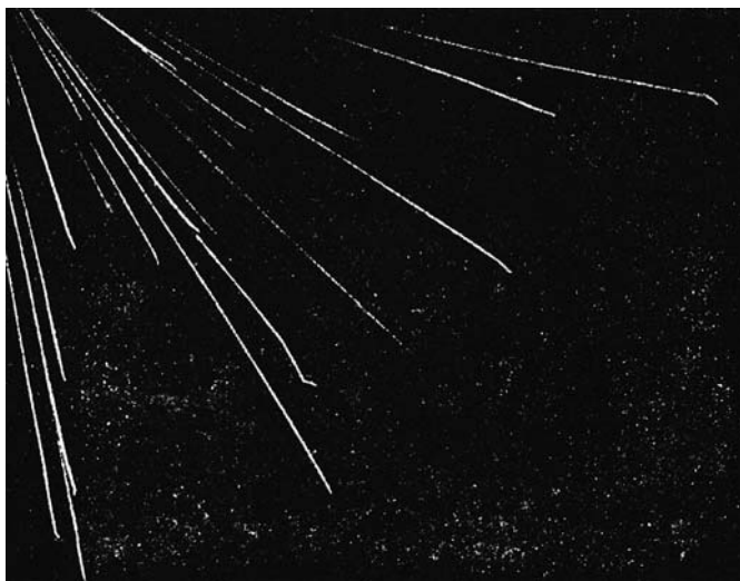
Figure 5.1. Tracks of alpha particles formed in a Wilson cloud chamber. (Adapted from W. Heisenberg, The Physical Principles of the Quantum Theory , Dover, New York, 1930, p. 5.)
