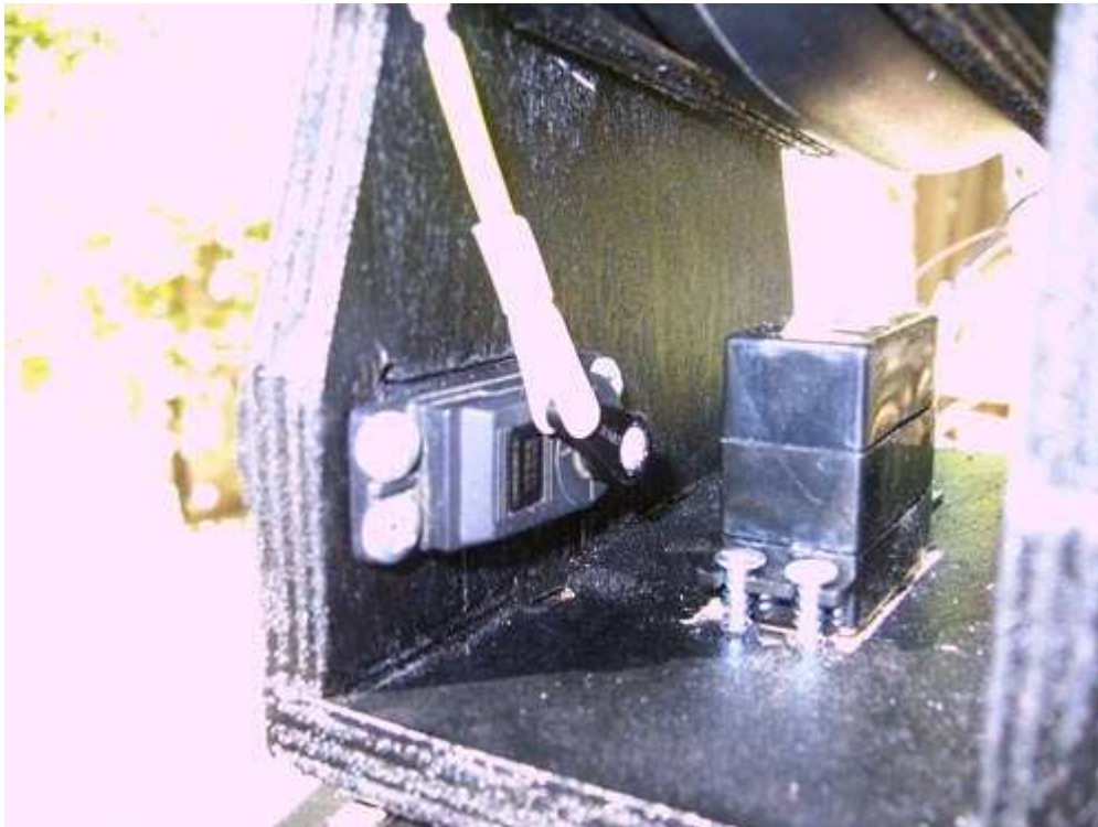
These are the pan and tilt control servos (on the painted turret). The one on the right is a direct drive servo that connects to the dowel in the middle of the lazy susan bearing. The servo on the left uses RC airplane elevator linkage to connect to the tilt head. The control software for the latter was more difficult to program because it's actually a four-bar linkage, and I am not a mechanical engineer. This was the simplest explanation of how to calculate input and output angles in a four-bar linkage, if you're interested.
