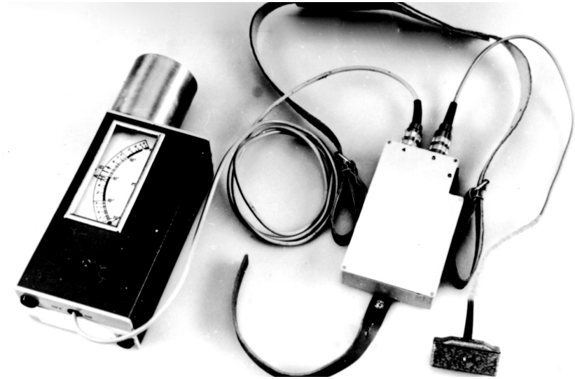
32. “Cloud 005” – a scintillator nuclear detection instrument. The device is on the left, and the battery pack, with the vibrating signal alarm attached, is on the right. (BStU)
