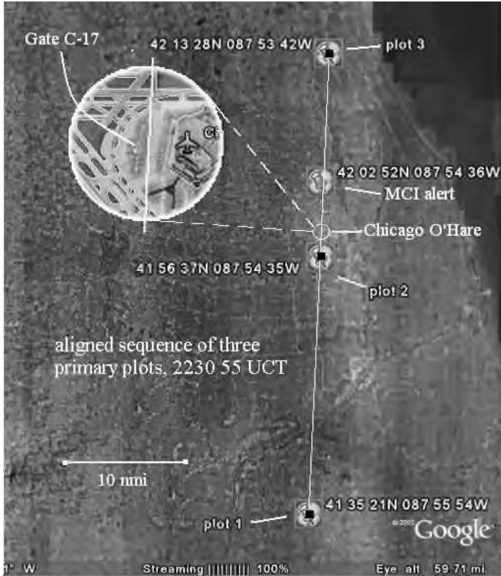
Fig. 30 Alignment of 3 Primary Radar Plots at 2230:55
