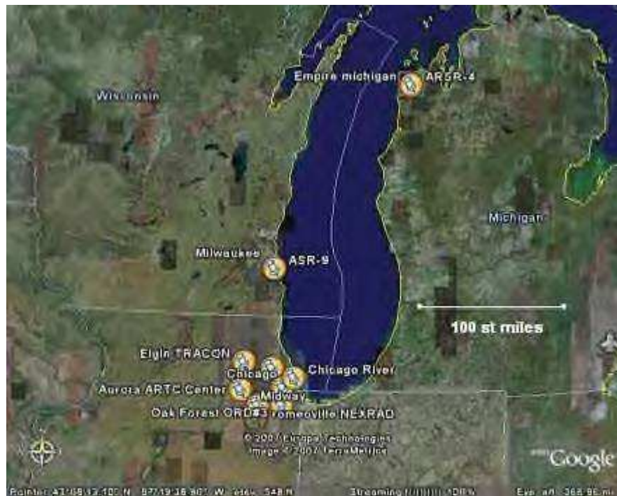
Figure 18. Radar Locations Around Lake Michigan Showing the ARSR-4 at Empire, Michigan, and ASR-9 at Milwaukee. The maximum range of the latter falls a few miles short of the area of the incident at Chicago O'Hare.
