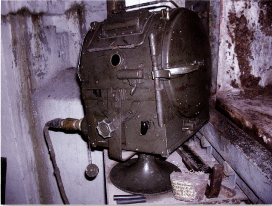
An AEG electric searchlight. The brightness could be controlled by adjusting the distance between two carbon rods through which an electric arc passed. A mirror in the back of the housing increased the brightness and the light could be focused with a powerful lens. (Author's collection)
