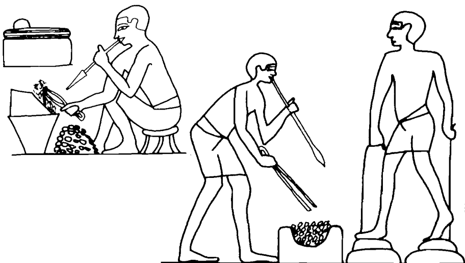
31. (Left) A smith works at a brazier to anneal a metal object. (After Davies, The Tomb of Rekh-Mi-Re at Thebes , New York, 1943, plate 55.)
