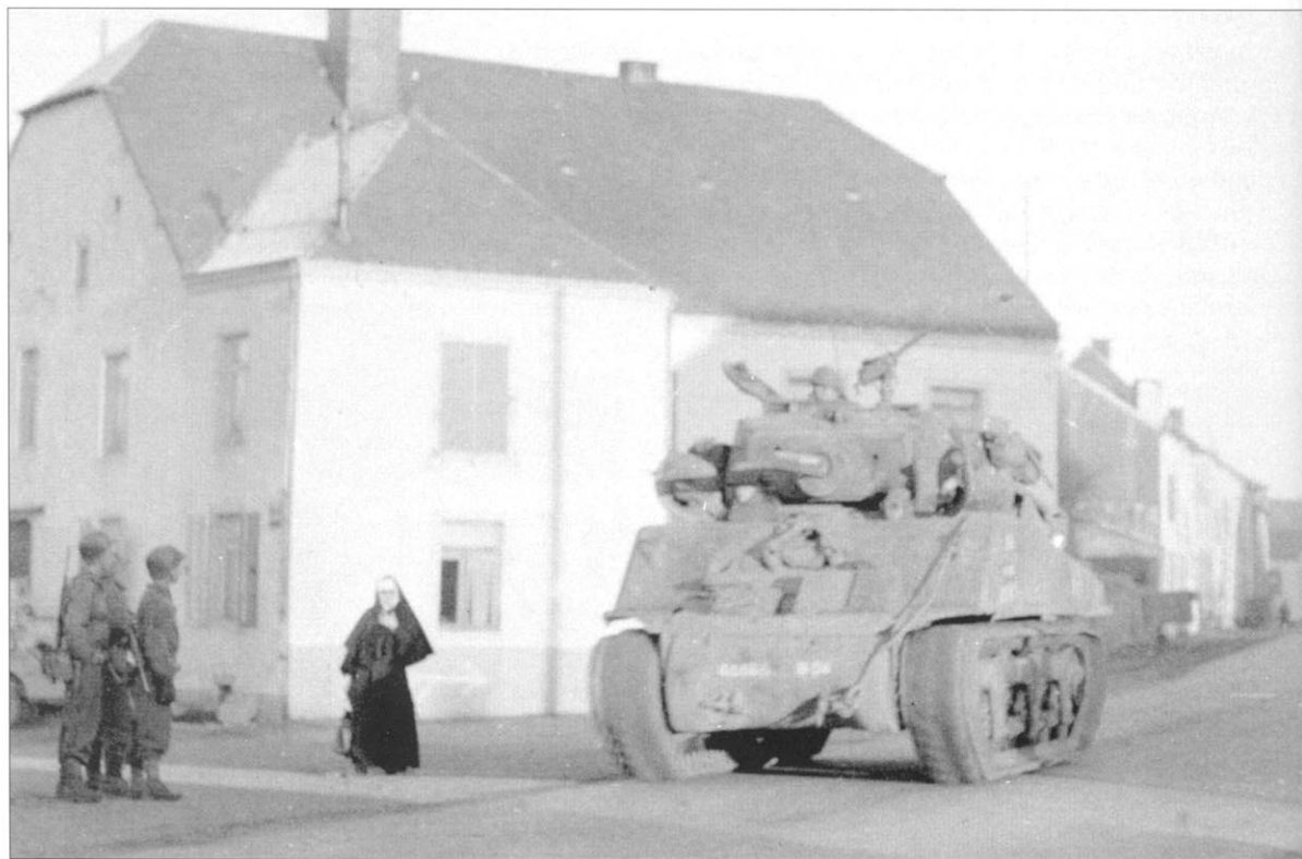
On New Year's Day 1945, 6th Armored Division was assigned to regain the initiative for Patton's Third Army in the attempts to breakout from Bastogne and link up with the First Army around Houfallize. This is an M4A3E2 assault tank of Co. B, 68th Tank Battalion, 6th Armored Division, passing through the town of Habay-la-Neuve on December 29 on its way to this assignment. (US Army)
