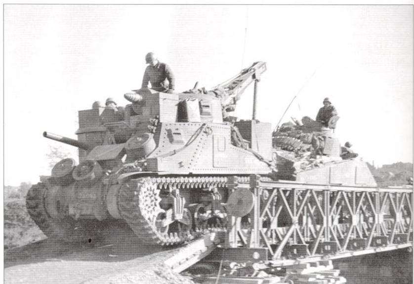
Armored divisions in 1944 were supposed to be equipped with the M32 tank recovery vehicle but in fact many still used the older M31 TRV, like the one seen here named "Invader" from the maintenance section of Co. I, 66th Armored Regiment, 2nd Armored Division, towing a damaged M4 medium tank over a Bailey bridge near Palenbourg, Germany, on October 15, 1944. (USMA)
