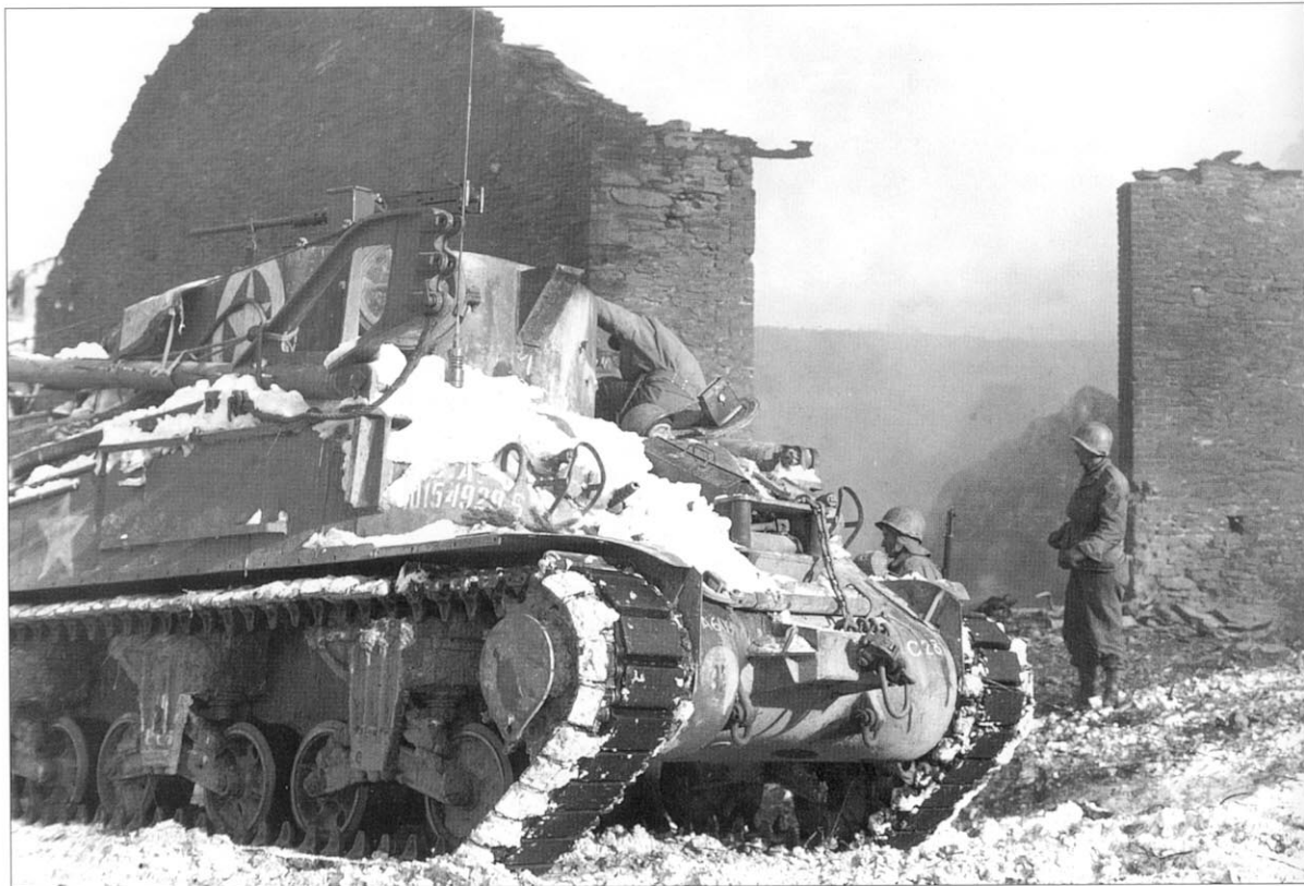
The principal tank recovery vehicle of the armored divisions in the ETO was the M32, based on various versions of the M4 medium tank. This particular example is an M32B1, based on the M4A1 chassis and is seen here supporting the 6th Armored Division in operations near Bastogne on January 14, 1945. (US Army)
