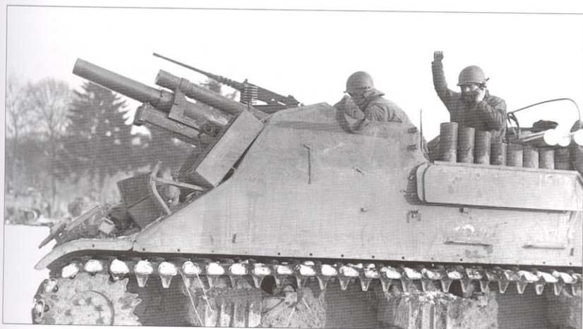
The workhorse of the armored field artillery battalions was the M7 105mm howitzer motor carriage. The crew of an M7 105mm HMC of Battery C, 274th Armored Field Artillery Battalion, prepare to conduct a fire mission in support of Patton's Third Army near Bastogne on January 1, 1945. The side armored flap is folded down, showing the tops of the fiberboard ammunition canisters in the ammunition racks along the side of the vehicle. (US Army)
