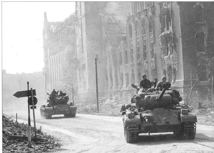
A small number of the new T26E3 heavy tanks arrived in the ETO and saw combat starting in March 1945. This is a pair from the 2nd Armored Division passing through Magdeburg after the intense fighting for the city in the middle of April 1945. (US Army)
