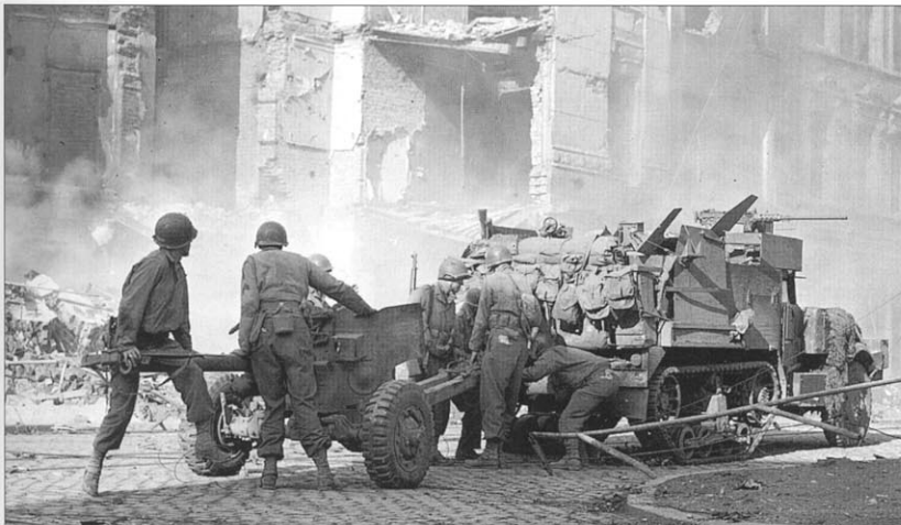
Anti-tank defense in the armored infantry companies was provided by the M1 57mm anti-tank gun, a license-built version of the British 6-pdr. With the advent of more heavily armored German tanks like the Panther, this gun was obsolete. Each armored infantry company had an anti-tank platoon with three of these guns, usually towed by the M2A1 half-track car. Here, a gun crew is seen unlimbering a 57mm gun from its half-track during the fighting in Aachen on October 15, 1944. (US Army)
