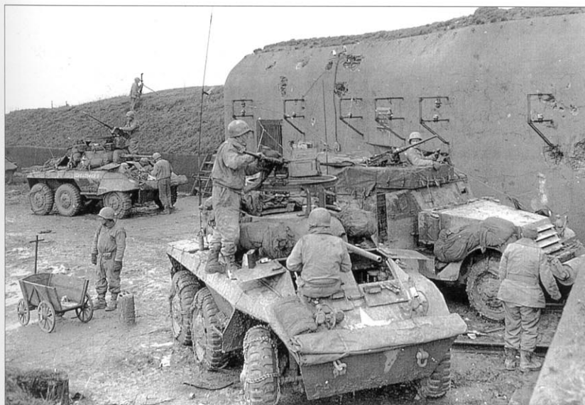
The workhorse of the cavalry reconnaissance squadrons was the M8 light armored car. An M8 armored car troop from the 92nd CRSM, 12th Armored Division, is seen here using an abandoned fortress from the Maginot Line near Guising, France, for a bivouac on December 13, 1944. Half-tracks, like the M3A1 here, were used in the squadron's maintenance and supply sections. (US Army)
