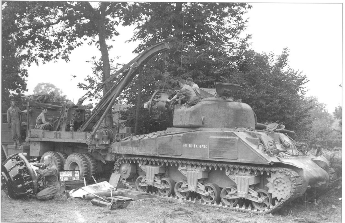
The tank battalion was organized to operate autonomously and perform its own basic maintenance. Here, an M1 heavy wrecker replaces the Continental R-975 radial engine in a M4 medium tank of the 2nd Armored Division during Operation Cobra on August 16, 1944, near Le Teilleul, France. (US Army)
