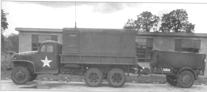
Each armored signal company deployed a high-powered radio section with six SCR-299 radio stations. This consisted of a 2½-ton truck with a HQ-17A shelter, and a semi-trailer carrying the PE-95 power generator. This basic configuration was used with other high-power radio stations such as the SCR-399, which shared some common components such as the BC-620 transmitter. (US Army)
