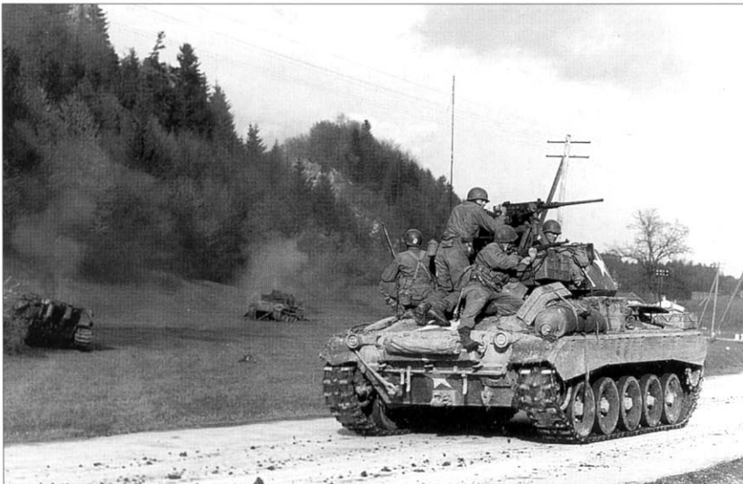
An M24 light tank of the 20th Armored Division with infantry aboard rolls past the smoking wrecks of a pair of Bergepanther armored recovery vehicles in the outskirts of Salzburg, Austria, on May 4, 1945, in the Seventh Army sector. Some of the new armored divisions had their light tank companies equipped entirely with this new type when they were deployed in the ETO in spring 1945. (US Army)
