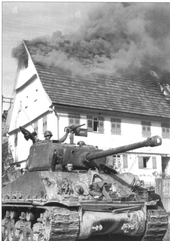
The ultimate version of the Sherman tank in US Army service during the war was the M4A3E8 which began appearing in combat in late December 1944. It introduced a new suspension system and wider tracks, giving the tank better mobility in muddy conditions. This example is with the 21st Tank Battalion, serving with CCA, 10th Armored Division, during the fighting in Rosswalden, Germany, on April 20, 1945.
