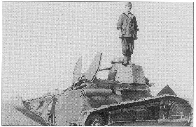
Soldier standing atop a Renault light tank to show the relative size of this small fighting machine. This machine mounted the 37mm gun. Others were armed with the Hotchkiss 8mm machine gun. This photo was taken at the US Tank Corps School at Bourg near Langres, France, in July 1918. American-built 6-ton tanks based on the Renault design did not reach France in time to enter combat. (US Signal Corps, 17546)
