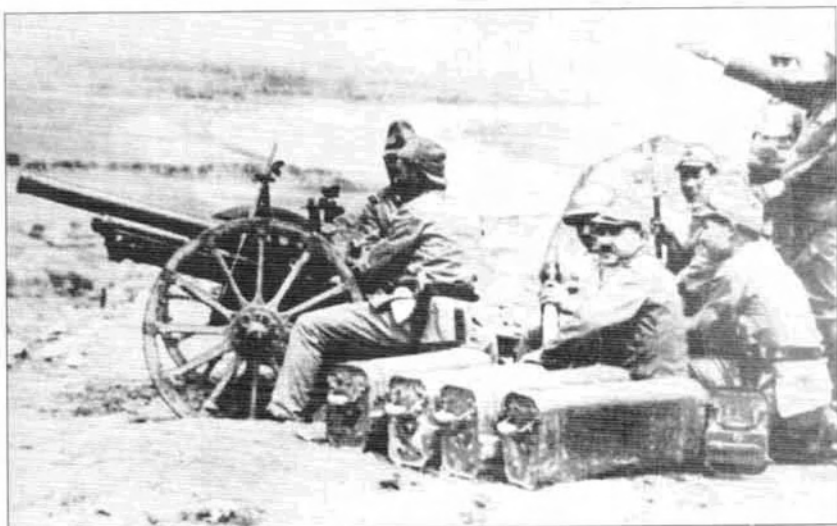
The 7.5cm Type 94 (1934) mountain gun weighed 1,200 lbs. It equipped half of the 12 divisional artillery regiments committed to the Southern Operations. The metal ammunition containers each held six rounds and weighed 118 lbs when full. A packhorse could carry two containers.
