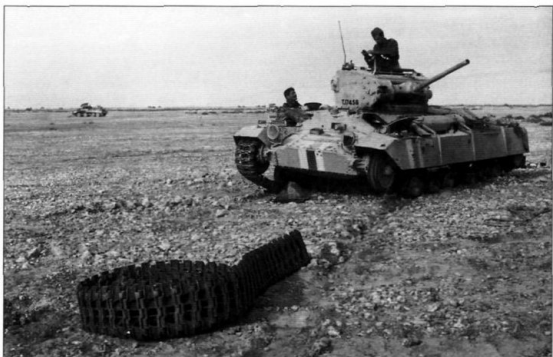
A Valentine tank which has thrown a track undergoing repairs in the Western Desert, 10 December 1941. (4700-32 E 7002)
