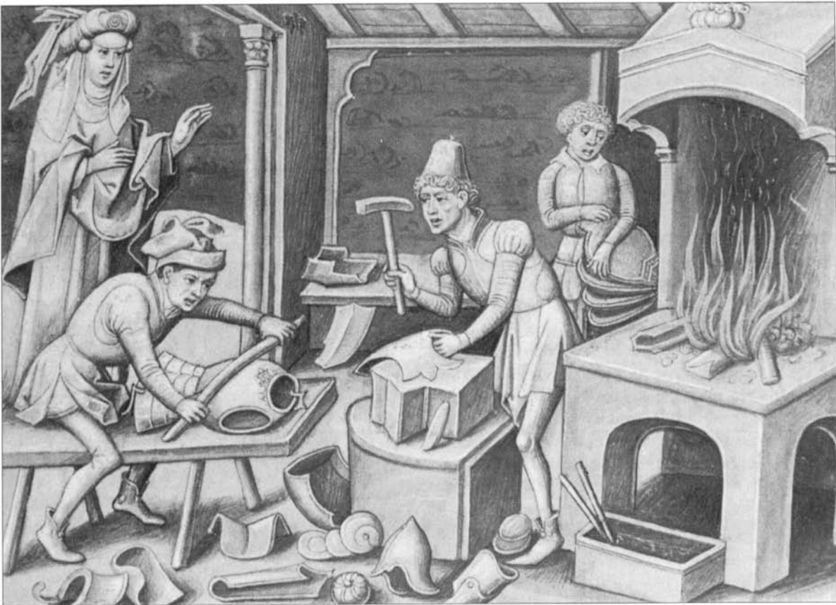
A grisaille of about 1460 by Guillaume Vreland shows an armorer cold hammering a plate while another burnishes a breastplate. (Friedrich-Alexander-Universität Erlangen-Nürnberg)
