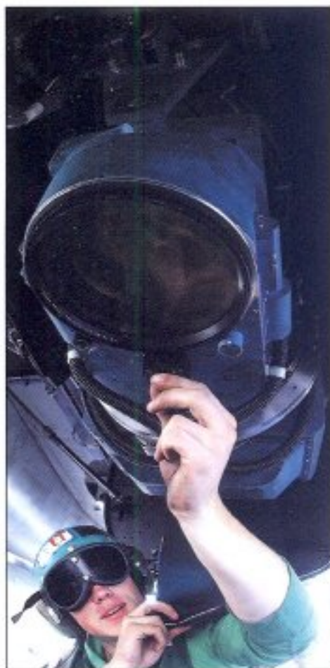
A photographer's mate from VF-41 adjusts the aperture on the lens of a KS-153B long-range camera. Of the three sensors fitted in the TARPS pod, the KS-153B was usually the most important. Following the pod upgrade in the early 1990s, the KS-153B was interchangeable with the older KA-99 low altitude pan camera (US Navy)
