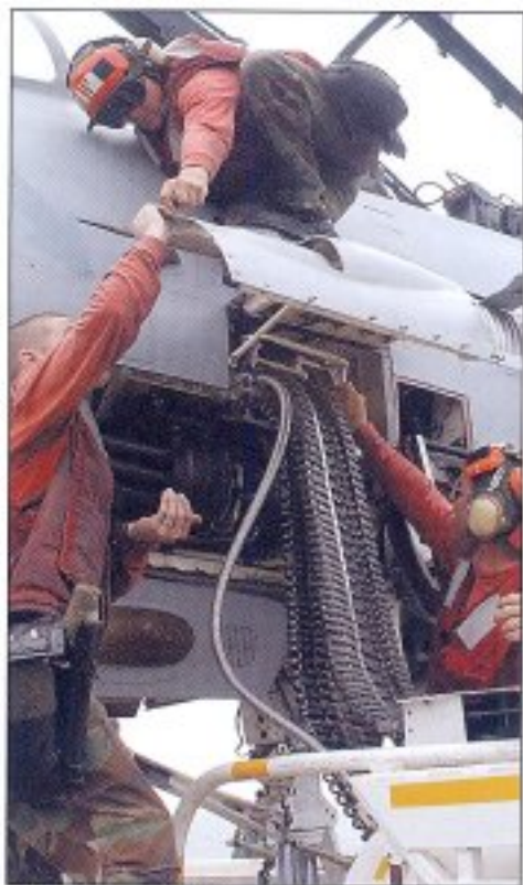
'Ordies' from VF-103 load 20 mm SAFHEI rounds into the magazine of an F-14B on the deck of CVN-73. A gun jam on 20 July 2002 ruined VF-103's one and only chance to see combat in OEF (US Navy)
