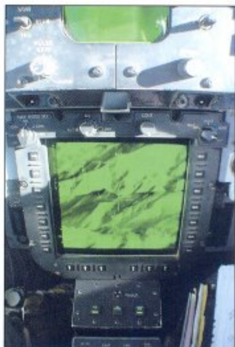
The large 8 x 8-inch PTID screen in the rear cockpit of a VF-102 F-14B reveals the rugged Afghan landscape near Tarin Kowt on 17 November 2001. This view, obtained via the LTS pod while circling the target area at 31,980 ft, could be panned in or out, depending on the mission requirements. No other TACAIR platform in OEF – Navy or Air Force – had a tactical display of this size, and when combined with the LTS pod, the Tomcat became the precision bomber and SCAR/FAC(A) platform of choice in-theatre (VF-102)
