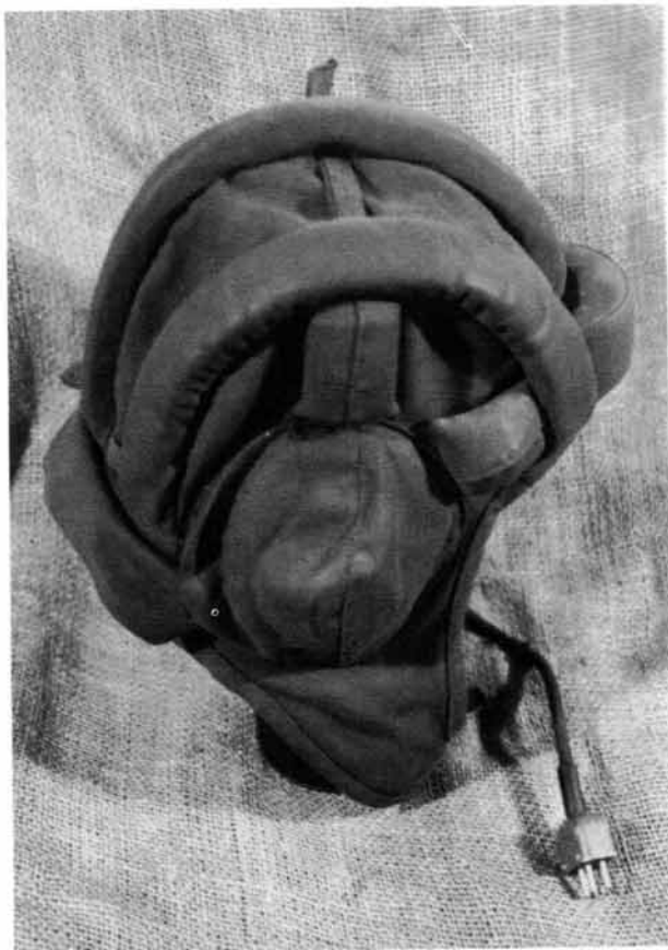
The standard summer tankers' helmet is similar to the Second World War version but has different ear guards for the intercom. Note the quick-attachment jack for the intercom system. (Author's photo)
