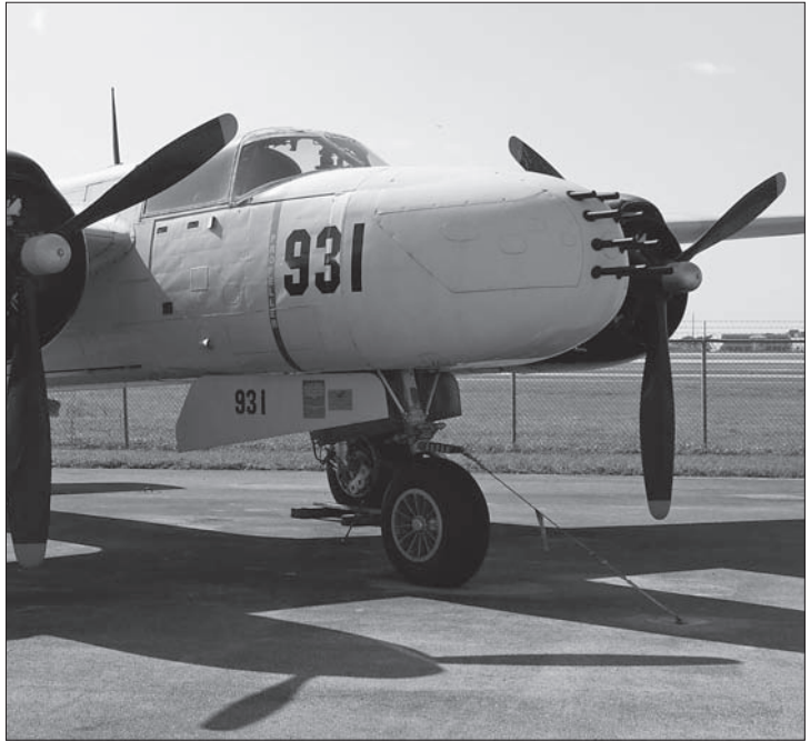
The "business end" of a Cuban-marked B-26B, showing its nose battery of eight .50cal machine guns. The pretence that the preliminary air strikes on April 15 had been carried out by defecting pilots from Castro's air force was not helped by the fact that the Brigade's invaders were the metal-nosed B-model, while those of the Fuerza Aerea Revolucionaria were C-models with a plexiglass nose for a bombardier. (Author's photo)
