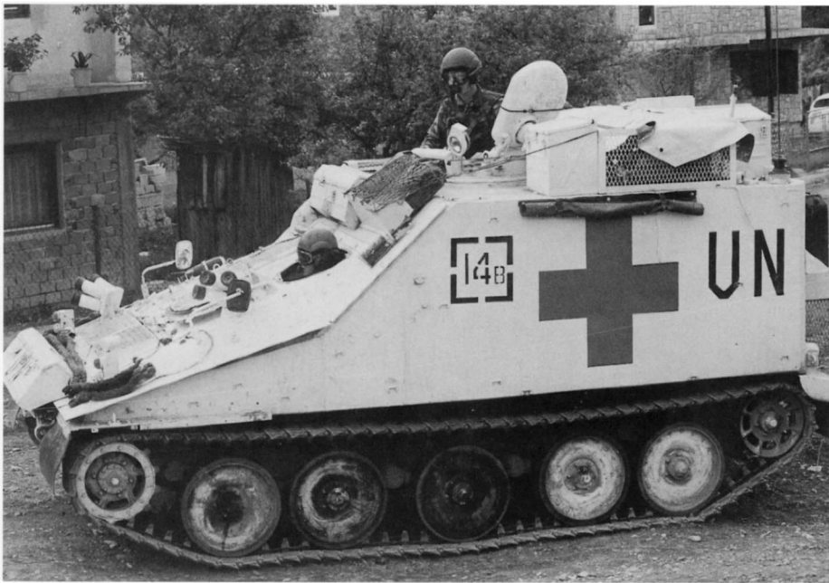
Samaritan is the armoured ambulance variant of the CVR(T) family and is designed primarily for casualty evacuation from forward battle areas. The first prototype was completed in 1973 with the first production vehicles being delivered in 1978. Here, callsign Fourteen Bravo, a Samaritan of Squadron Headquarters, 'B' Squadron, The Light Dragoons, provides medical cover during Operation 'Cabinet' on 19 May 1993 when a major UNHCR convoy from Belgrade was escorted by The Light Dragoons over the Bosnia/Serbia border. (MoD P.Info UKLF)
