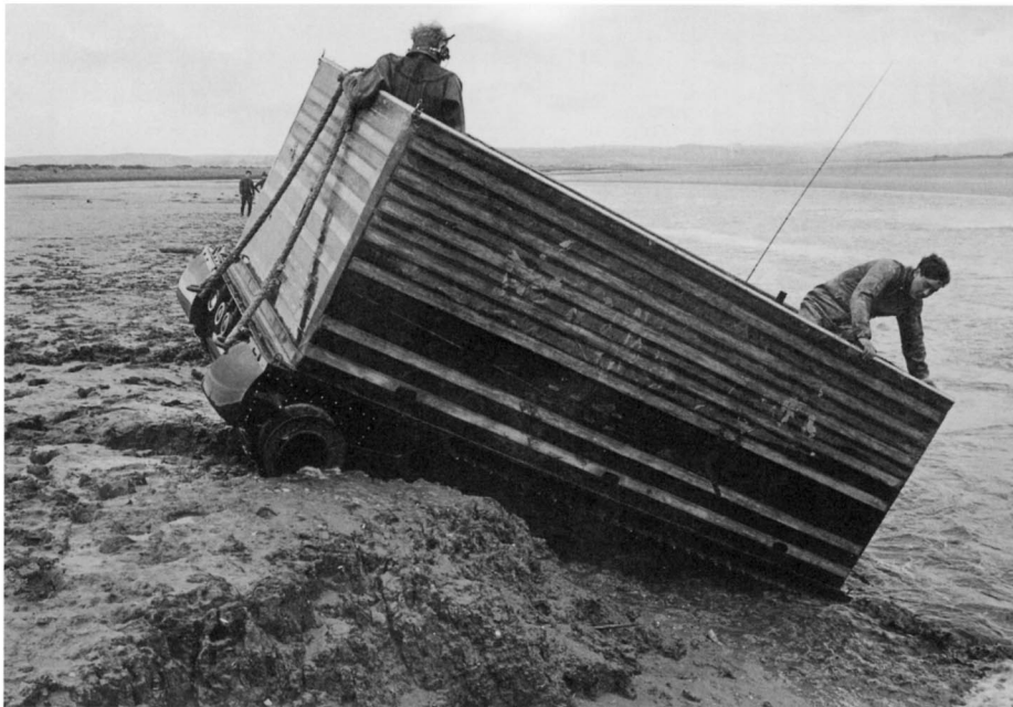
A prototype Scorpion, recognisable by the additional pair of headlights fitted with IR filters, undergoes wading trials to test its amphibious capability. The collapsible rubberised floatation screen of CVR(T) can be erected in under ten minutes and allows the vehicle to negotiate still rivers and waterways at speeds of up to 3.6 mph (6 km/h) while the generous freeboard of this system allows even steep-sided river banks to be negotiated on entry and exit. (Alvis)
