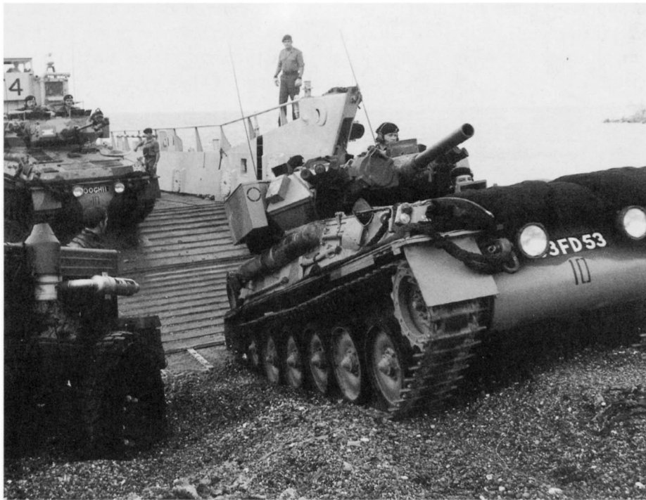
Sergeant Mouse directs his Scorpion of 'C' Squadron, 16th/5th The Queen's Royal Lancers, from an LCT of HMS Intrepid during a beach landing exercises at Lulworth in 1981 – the year that wading screens were removed from CVR(T). This Scorpion and Scimitar are assigned to ACE Mobile Force (Land) and are painted in the yellow and green camouflage scheme applied for service on the southern flanks of NATO in either Greece or Turkey. Both these vehicles have been fitted with the 7-in. headlights of Ferret and Saladin in place of the 5-in. Sealed beam units which proved to be less durable. (MoD)
