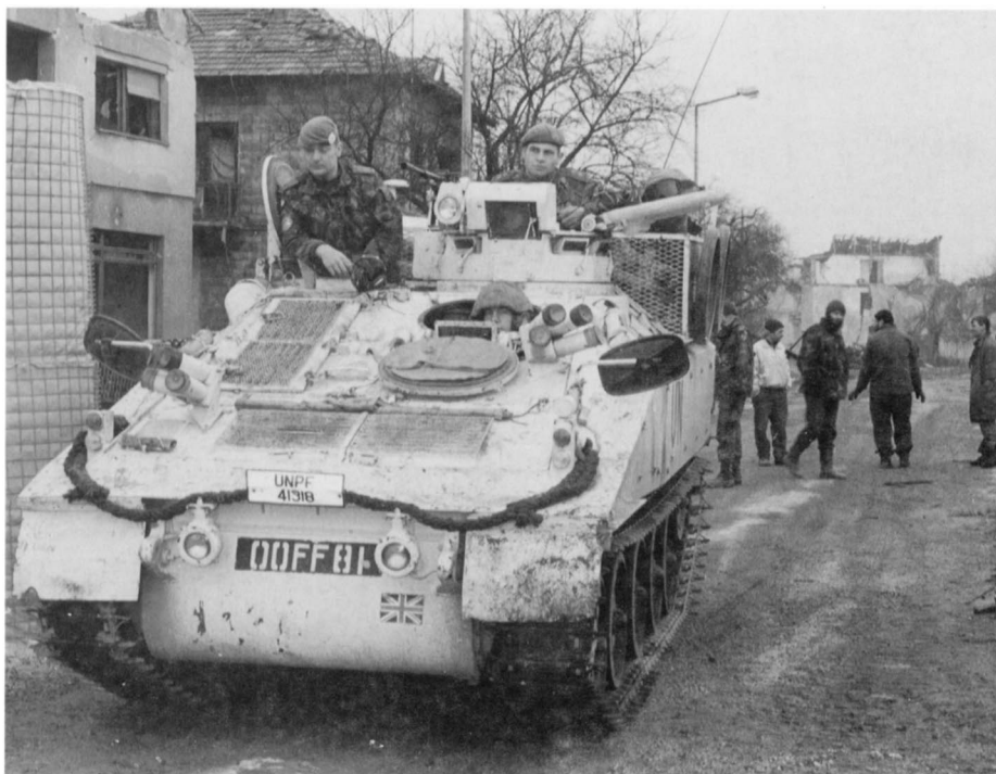
A Spartan of 'C' Squadron, The Light Dragoons, acts as a checkpoint near Zepce in March 1994. Because of its less aggressive appearance than Scimitar or Warrior, Spartan enjoys more flexibility of movement in disputed areas, being employed for numerous tasks such as the movement of casualties or VIPs. Note that this Spartan has the larger Samson-type rearview mirrors. A common modification to CVR(T) in Bosnia is the fitting of a metal stanchion above the hull or turret to cut wires strung across the road that otherwise could decapitate the crew members. (MoD P.Info UKLF)
