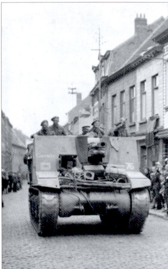
Sexton self-propelled gun of G Battery, A Troop, RHA (HAC), of whom Sergeant Saunders was the No.1. The gun was photographed in Belgium on its way to Antwerp in 1945. The number 76 is the arm of service marking for artillery. (Author's photograph)
