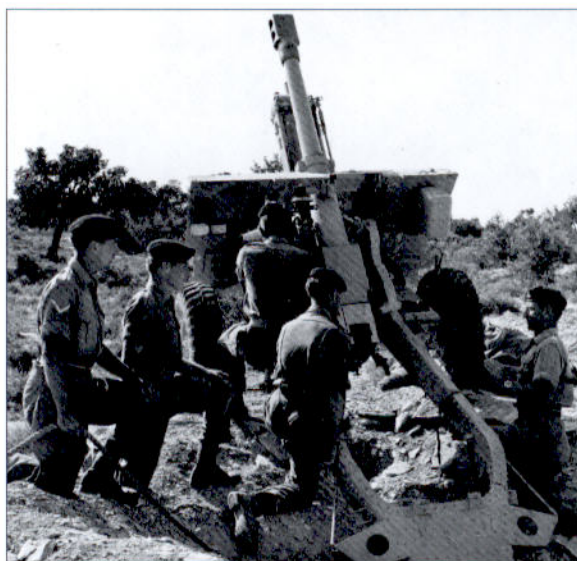
A 25-pounder of 42nd Field Regiment in a post-war role, possibly in the Middle East. The gun trail has been dug into a pit and hence the piece has a much higher elevation than on normal ground. The No.1 has a short rammer in his hand, intended to assist the shell into the chamber. (Courtesy of RAHT)
