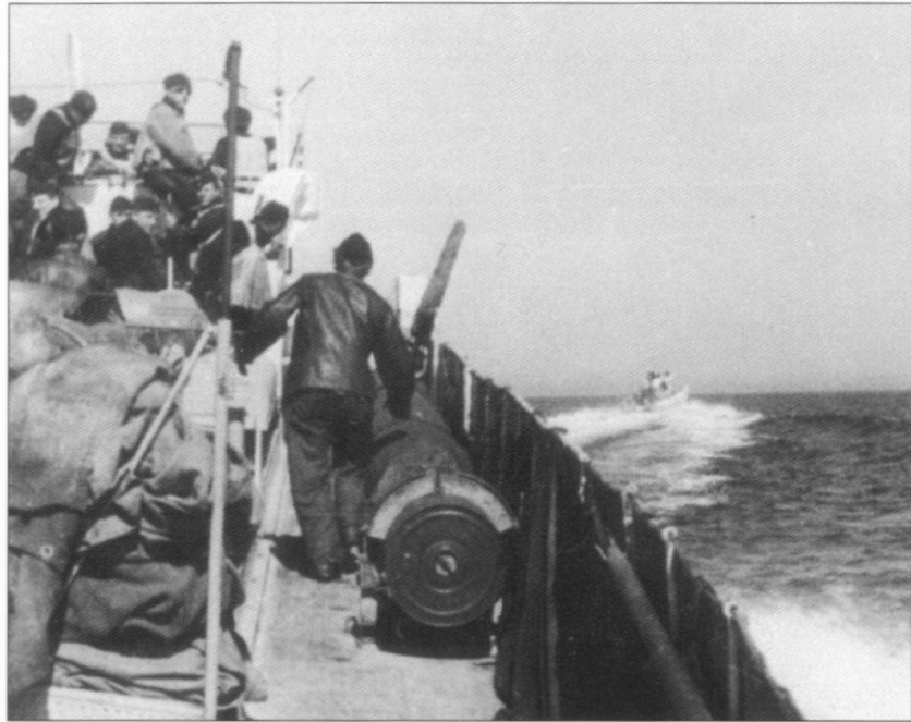
A view taken looking forward from the quarterdeck of an E-boat moving at some speed. The extreme slope of the deck is evident and must have made movement rather awkward to say the least. This boat seems to be carrying spare depth charges rather than torpedoes in the deck racks.
