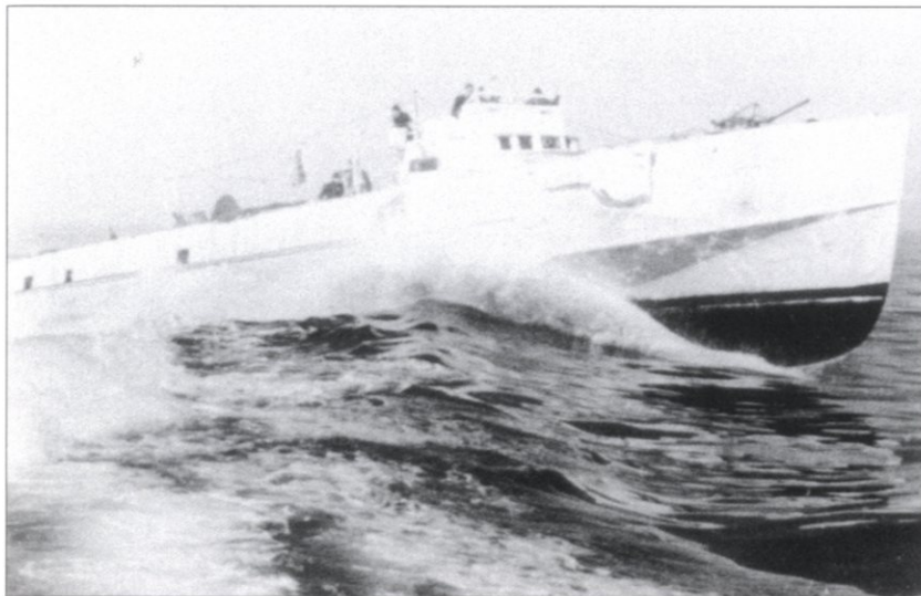
ABOVE Starboard view of a later-type high forecastle boat with 2cm bow gun and open bridge. Canvas dodgers have been fitted.
