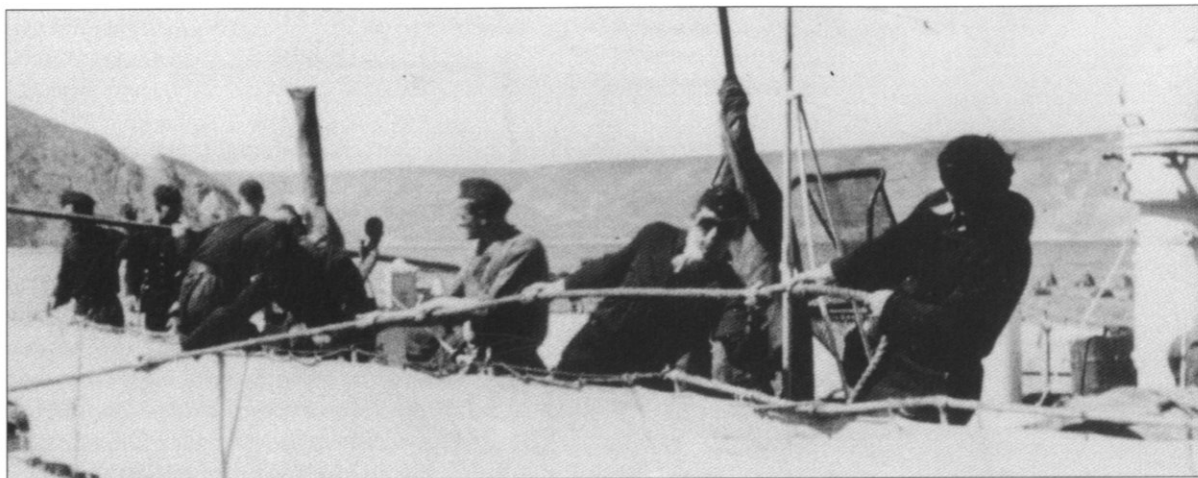
Crewmen pull the mooring ropes of their boat, drawing her into the quayside. This shot clearly shows the canvas dodger screens fitted over the boat's railing to avoid the afterdeck becoming swamped.
