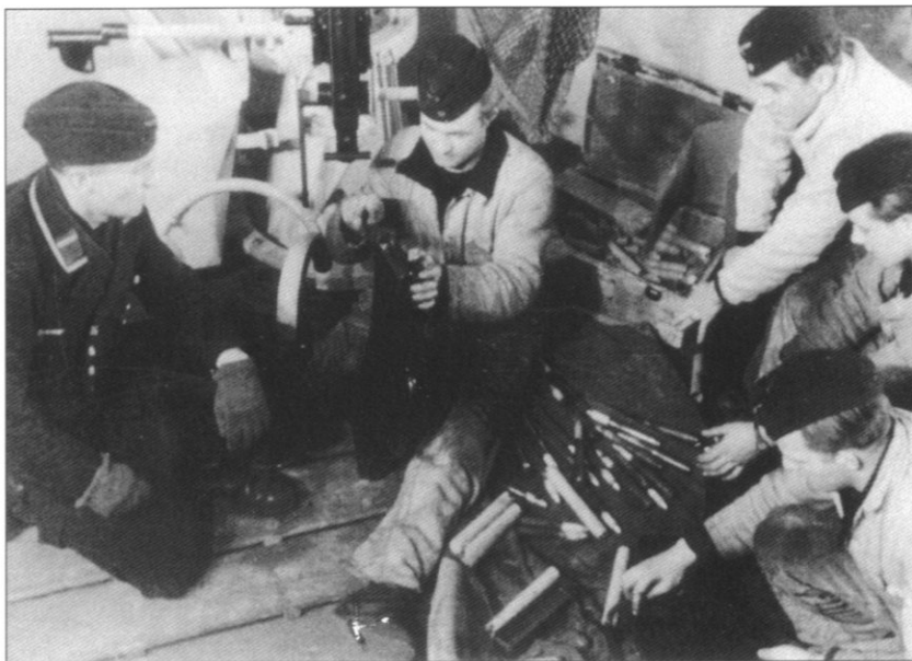
Watched by an attentive petty officer, and assisted by some of his crewmates, a sailor loads shells into a magazine clip for the 2cm flak gun. The breech of the gun can be seen just by the crewman's right shoulder. Note the shells lying on the canvas sheet by his left leg.
