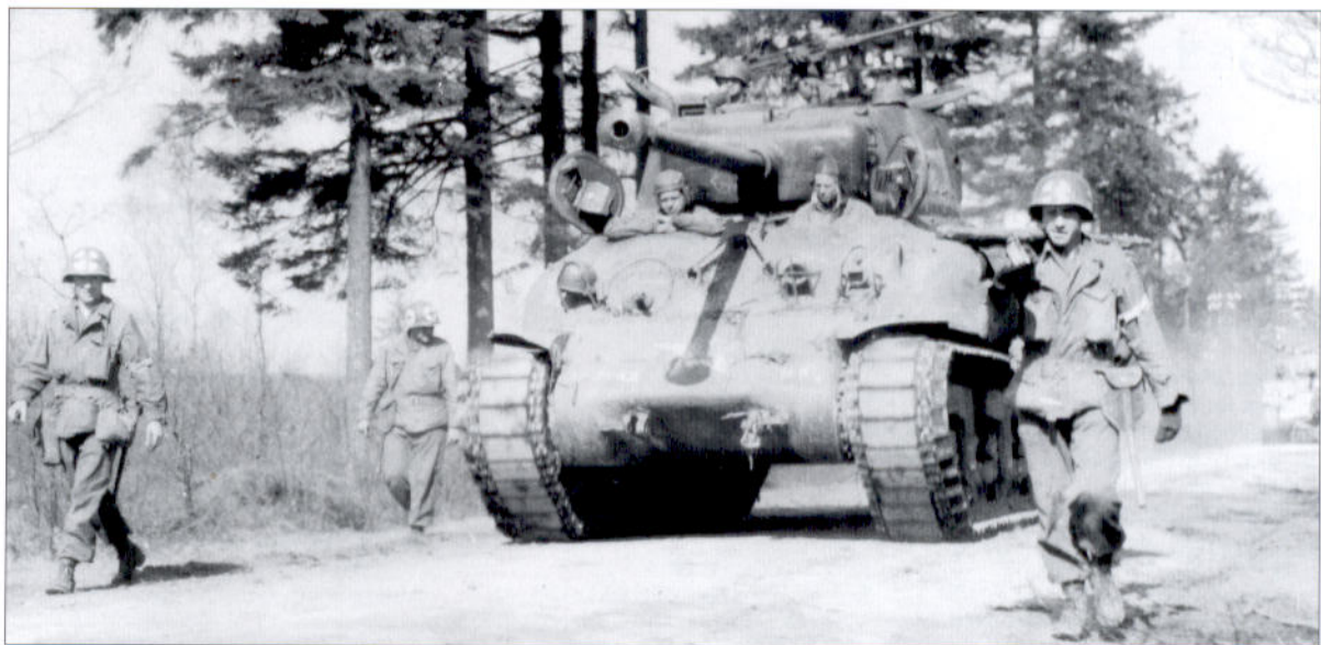
ABOVE Although nearly all M4 (76mm) tanks issued in the ETO after July 1944 were based on the M4A3 chassis, in the spring of 1945 some new production M4A1 (76mm) again appeared in the supply chain like this tank of Co. B, 774th Tank Battalion supporting the 78th Division near Honsborn, Germany, on April 10, 1945. They can be distinguished by the muzzle brake on the 76mm gun, not present on the small batch of M4A1 (76mm) issued in July 1944. (NARA)
