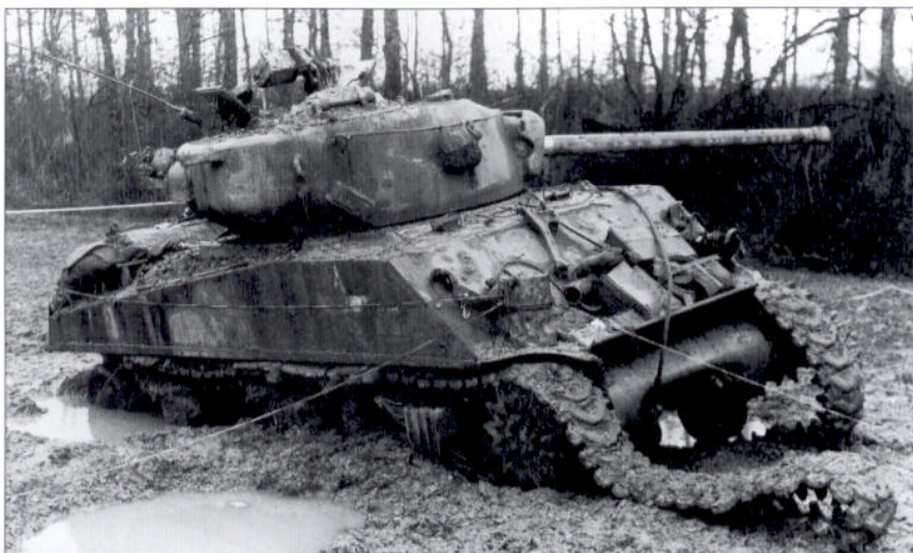
The autumn of 1944 was unusually wet in Belgium and along the German border, and the mud created a significant mobility problem for the M4A3 (76mm). This 6th Armored Division tank was knocked out near Hellimer, Germany, on November 25, 1944 after first striking a mine. (US Army)
