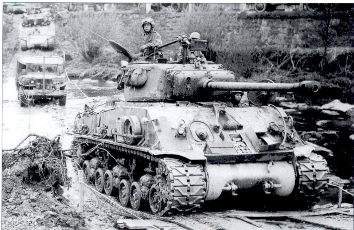
ABOVE Although nearly all M4 (76mm) tanks issued in the ETO after July 1944 were based on the M4A3 chassis, in the spring of 1945 some new production M4A1 (76mm) again appeared in the supply chain like this tank of Co. B, 774th Tank Battalion supporting the 78th Division near Honsborn, Germany, on April 10, 1945. They can be distinguished by the muzzle brake on the 76mm gun, not present on the small batch of M4A1 (76mm) issued in July 1944. (NARA)
