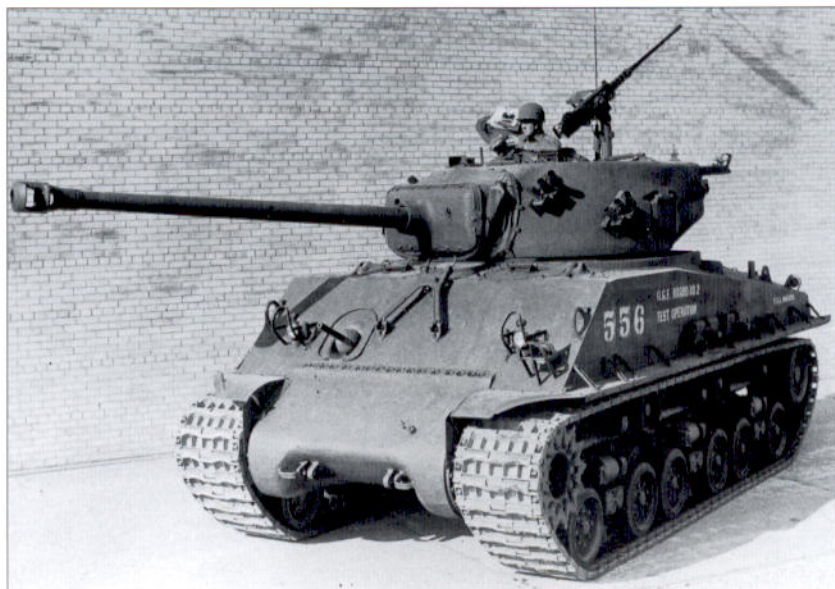
The ultimate solution of the mobility problems with the M4 tank was the 23-inch track, which was introduced into production along with the new HVSS suspension in August 1944. This M4A3E8 (76mm) is fitted with the initial T66 steel tracks and is seen during trials at Fort Knox. It is fitted with a set of experimental smoke dischargers on the turret side. (Patton Museum)
