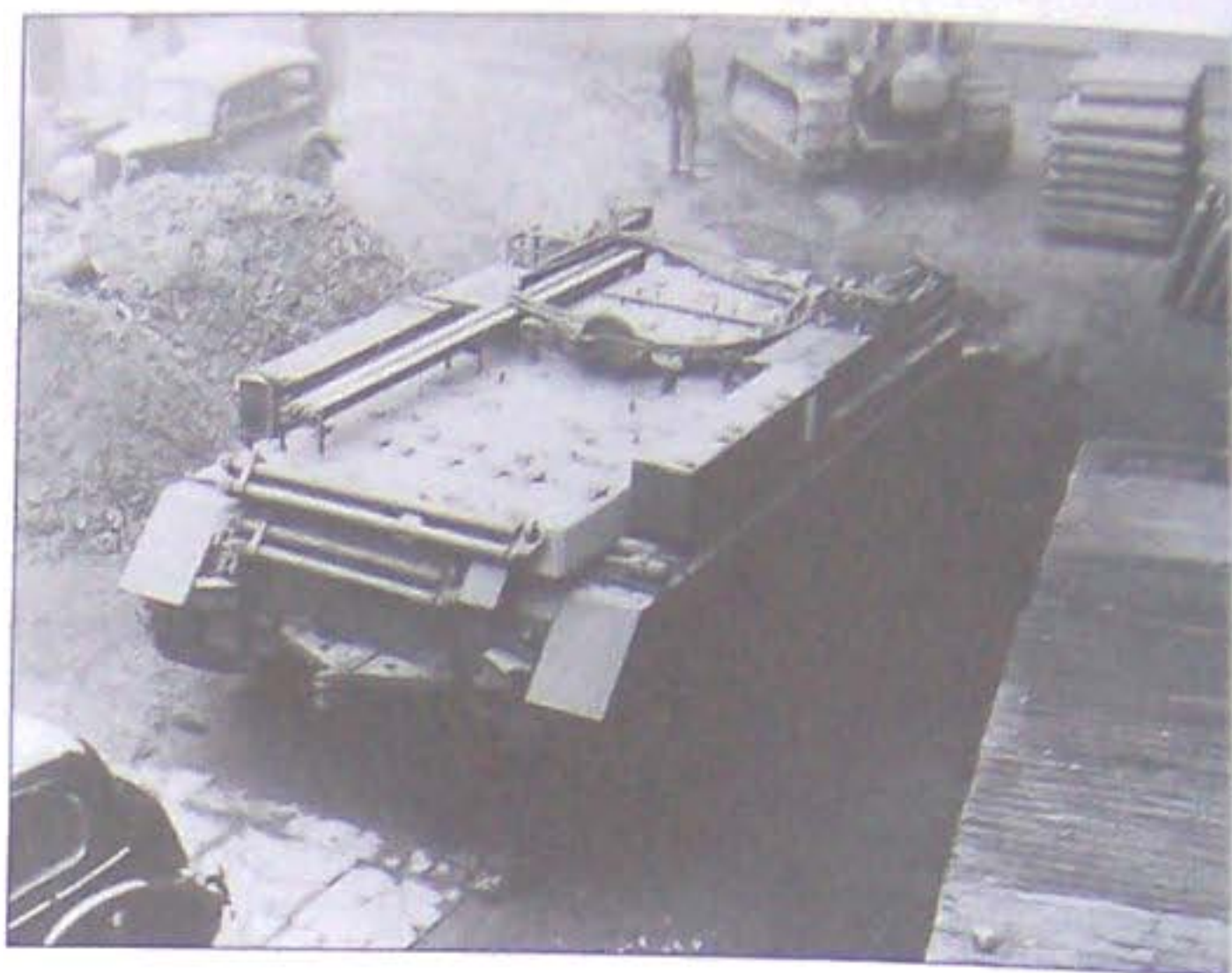
Fully stowed Cavalier ARV Mark I. Ahead of it the big Caterpillar D8 tractor represents an earlier period of tank recovery. Visible stowage includes Hollebone towing bars at the rear, front jib arms to the left and the tow cable with snatch blocks.
