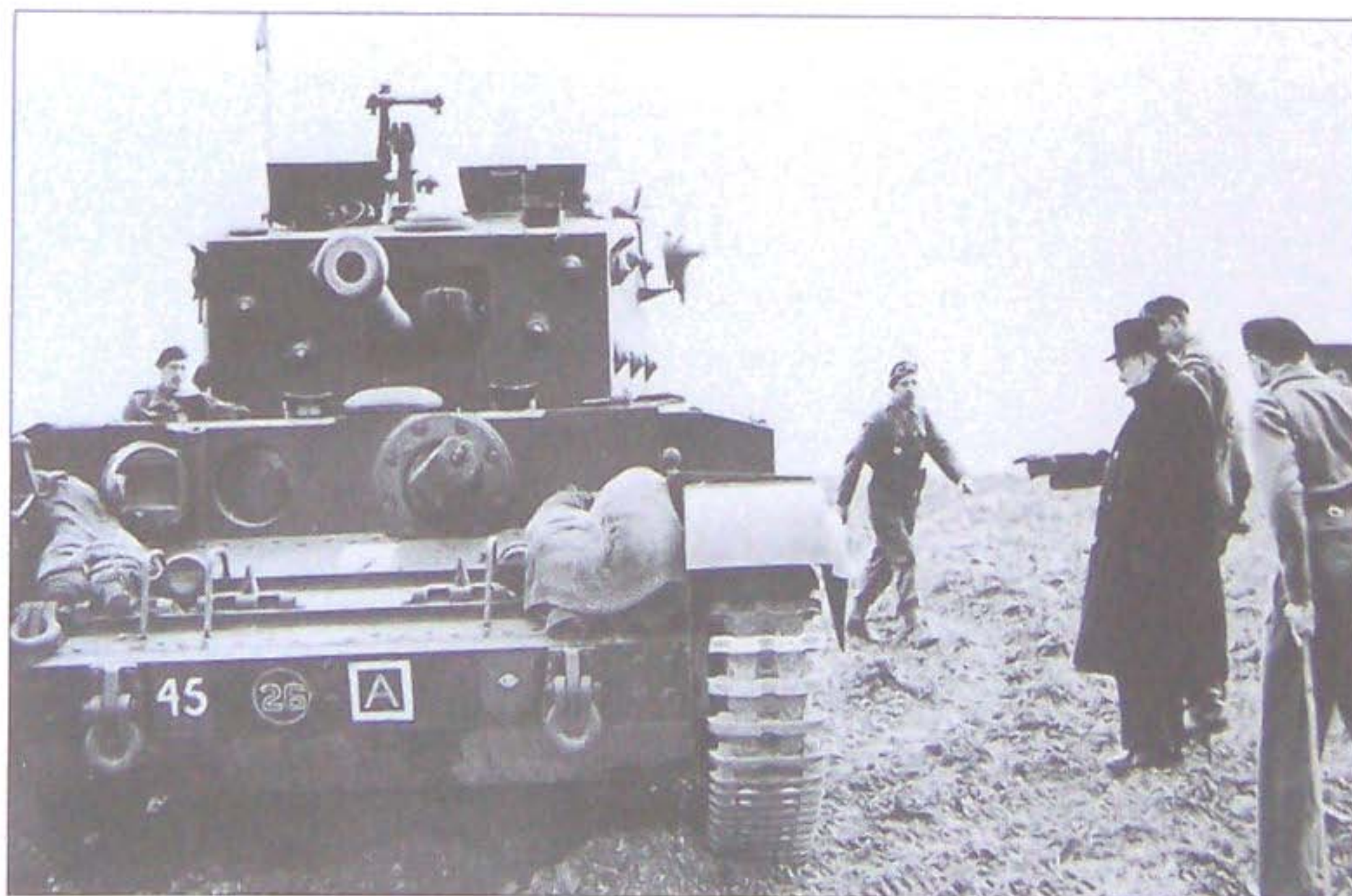
Winston Churchill is shown a Cromwell IV of No 2 Squadron, 2nd Welsh Guards, in March 1944. Notice how this regiment kept all markings as low down as possible, making them less eye-catching to the enemy. The aptly named Blenheim was the squadron commander's tank. The fitting on top of the turret is a PLM mounting, lacking its machine guns.
