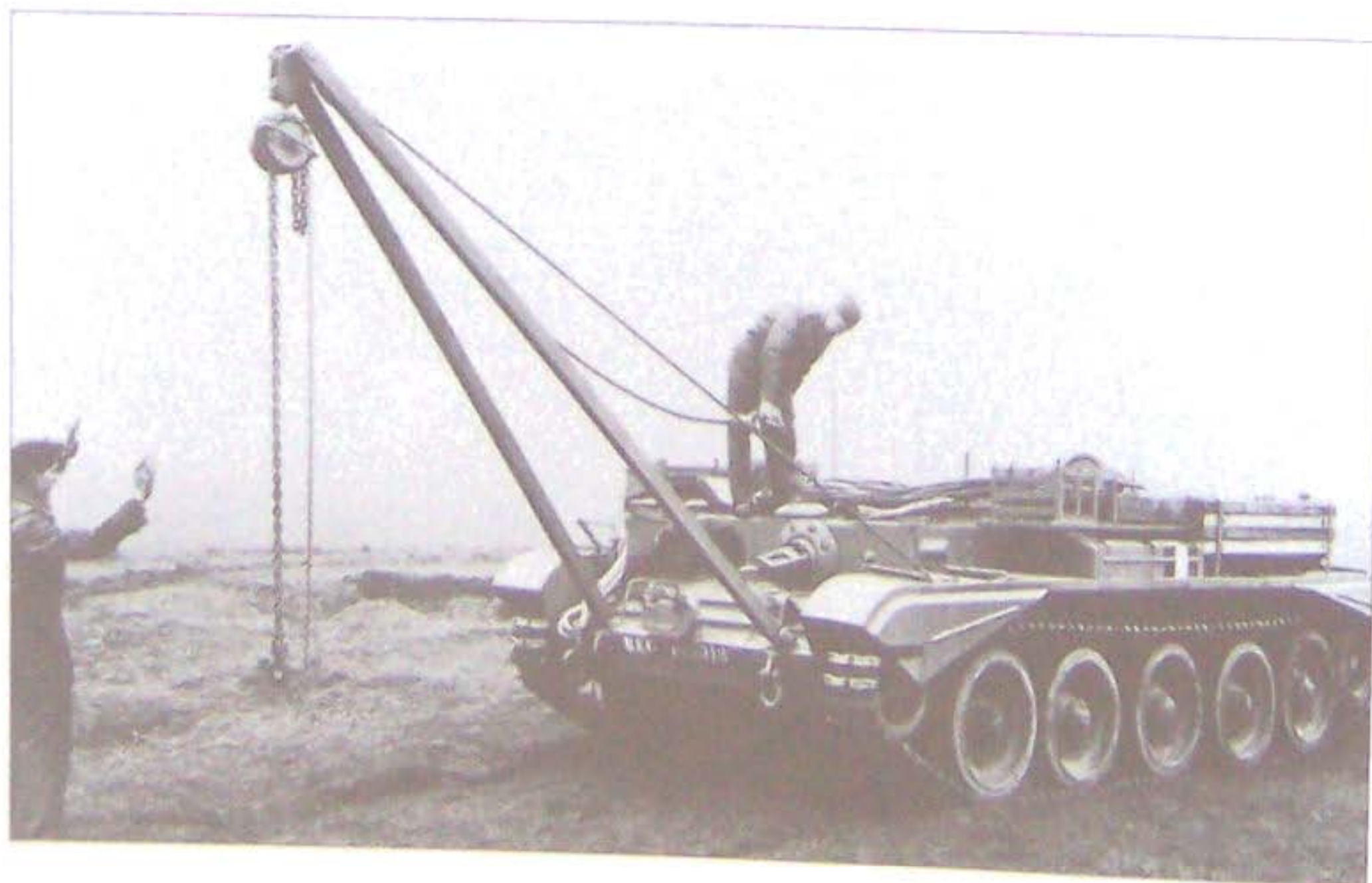
Raising the jib on a Cromwell ARV I. The tank reverses until the wire, linking track and jib, raises the latter in the correct place, when the man on top will secure the stay. A chain hoist is secured to the jib, there is a vict on the hull front and the BESA machine gun is still in place.
