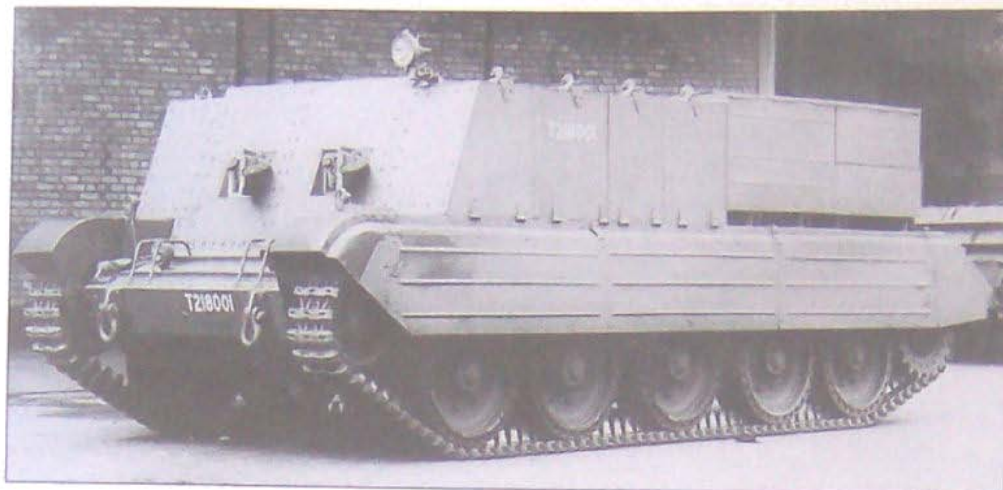
Centaur Taurus 17-pdr Gun Tractor, one of nine converted by MG Cars of Abingdon. The full-length sand guards were designed for Cromwell, but were very rarely seen on gun tanks.
