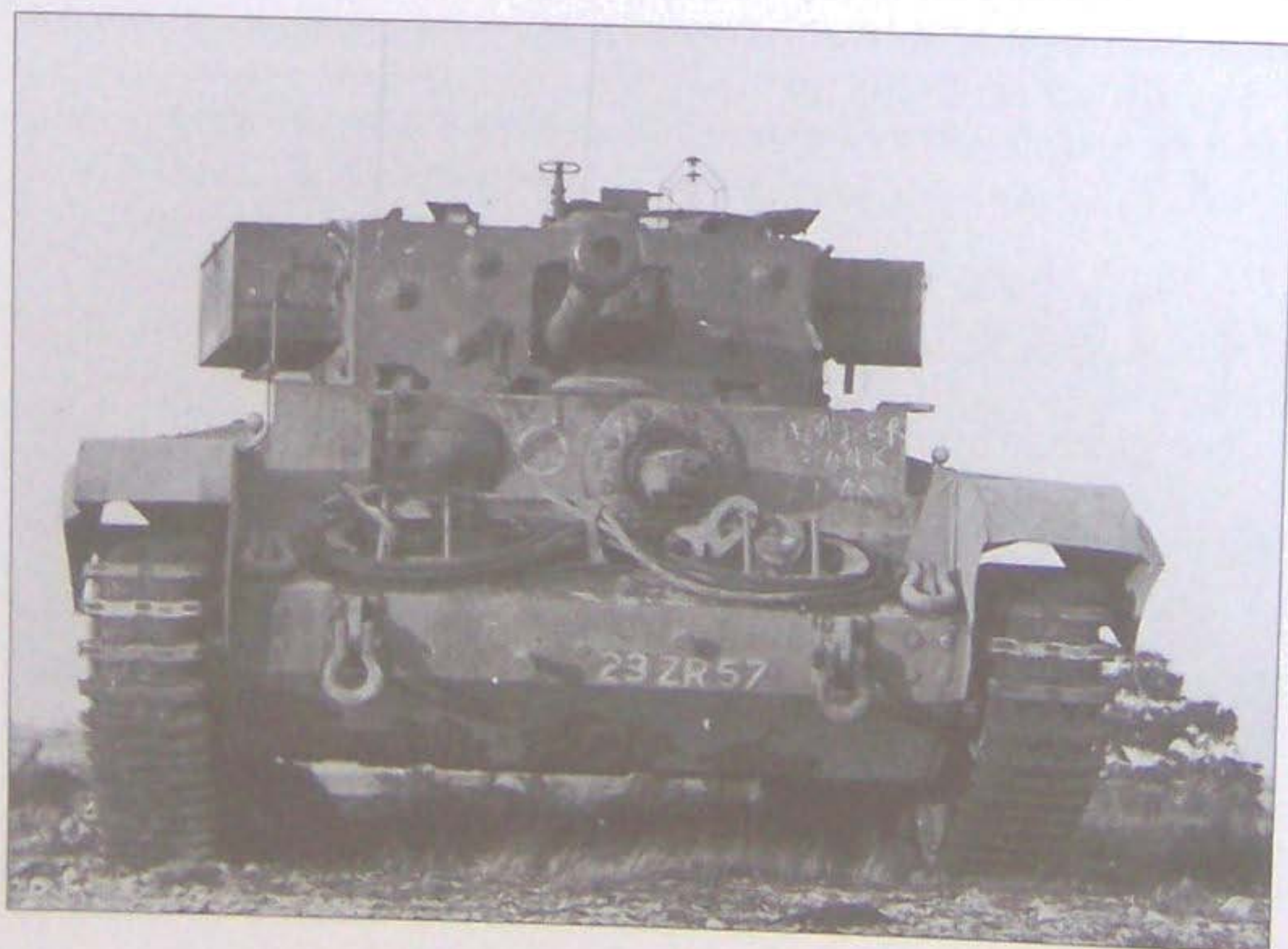
Although the vehicle here is in fact an OP tank, this photograph provides a good view of a Cromwell Mark IV with Type F hull in post-1948 condition. Prominent on the turret is the All-Round Vision cupola, late-style vane sight and turret stowage boxes.
