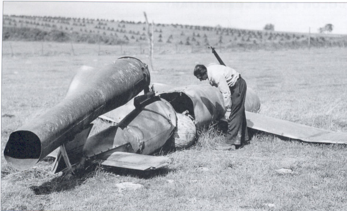
ABOVE This V-1 was one of many that prematurely crashed after launch in the French countryside, and is being examined by a member of the French resistance. The fuselage has split open behind the center fuel tank, exposing one of its two pressurized air bottles. (NARA)
