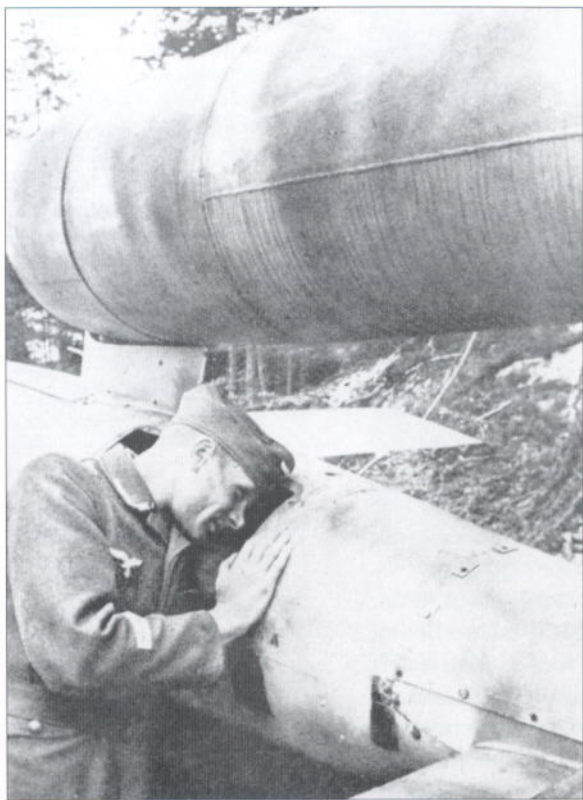
A member of the launcher section makes final adjustments to the missile autopilot assembly prior to launch. (NARA)
