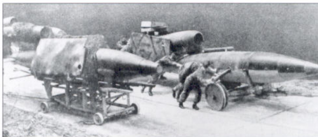
A supply battery of Flak Regiment 155 (W) prepares missiles for launch. The missile on the left is mounted on the Zubringerwagen loading trolley which was mated to the launch ramp, and the missile slid into place. (NARA)
