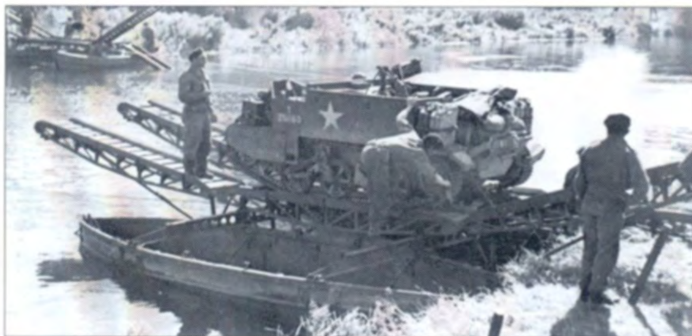
Polish troops and their Mark II MMG Carrier prepare for a ferry ride across the river Seine during the advance across France. The ferry, which is hauled across by cable, is assembled from lightweight trackway supported on two folding boat pontoons.
