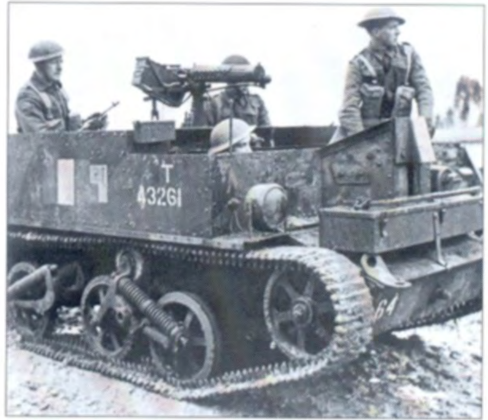
Canadian troops with an MMG Carrier in Italy, with the Vickers gun and ammunition box in place. T 43261 was a Canadian-built Mark I stripped of all tinwork but with personalized stowage arrangements and non-standard headlights. Red/white/red stripes on the side were an Allied identification sign in Italy.
