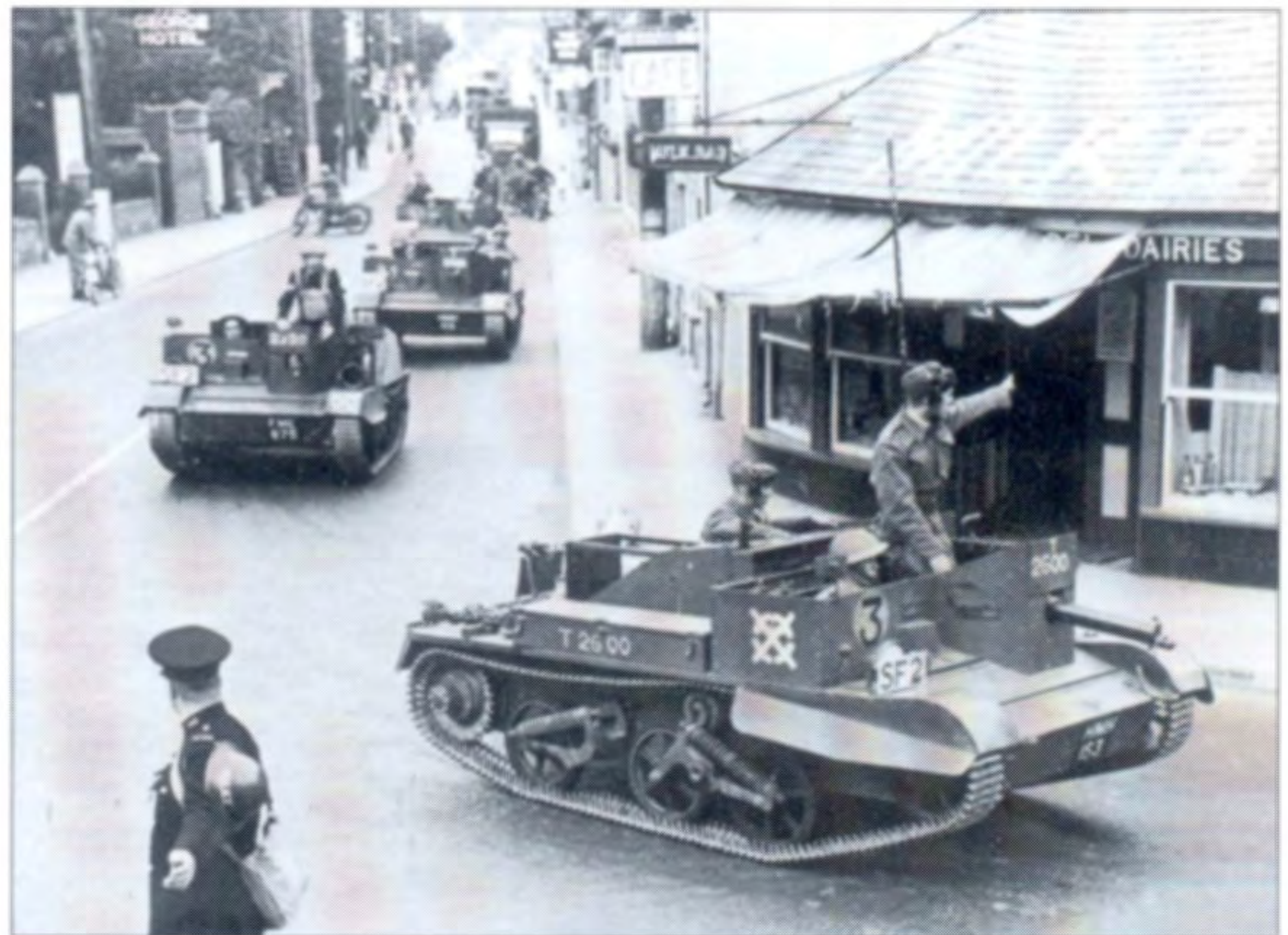
Not all of the Machine Gun Carriers No. 2 Mark II were rebuilt as Bren Gun Carriers when the war began. Here T2600, an early Thornycroft-built example, still features a Vickers gun in the enlarged gunner's compartment as it leads a column of carriers through Amesbury, Wiltshire. The markings suggest that they are playing the part of enemy vehicles in an exercise.
