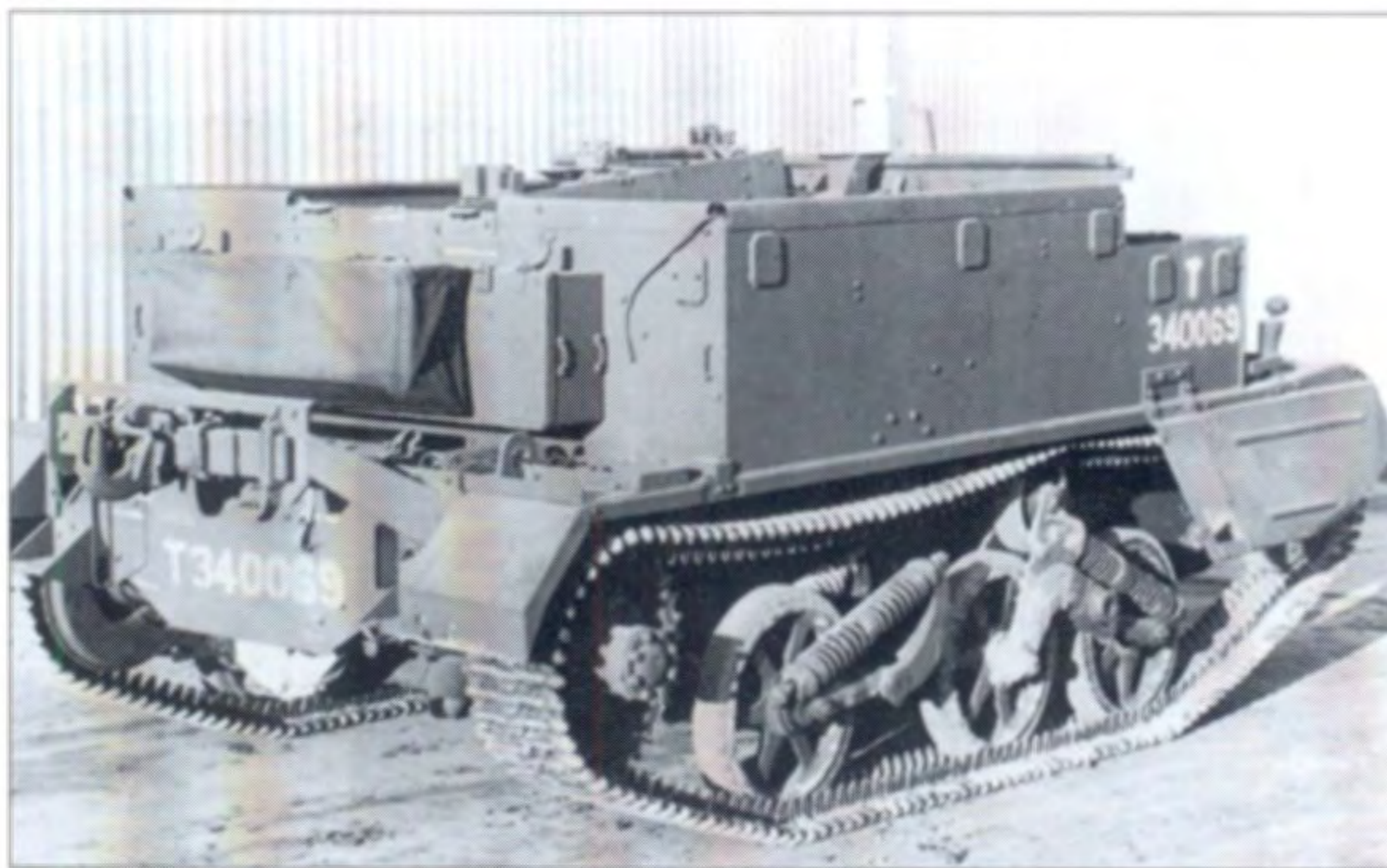
A Universal Carrier Mark III viewed from the rear shows the large stowage locker with the canvas holder attached, the strong Stacey towing attachment and the little square panels welded to the hull which are mounting points for the special deep-wading panels. The hull appears to be fully welded and it is finished off, around the top edge, by a simpler system of what appears to be thin plate, bent over.
