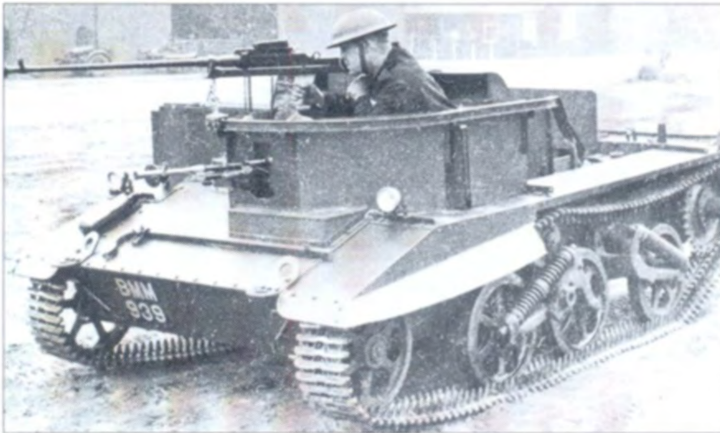
The only known photograph of the prototype BMM939 modified into the role of General Scout Vehicle. The gunner's compartment is much enlarged, with a Bren gun in the aperture and Boys anti-tank rifle on a sliding rail around the lip.
