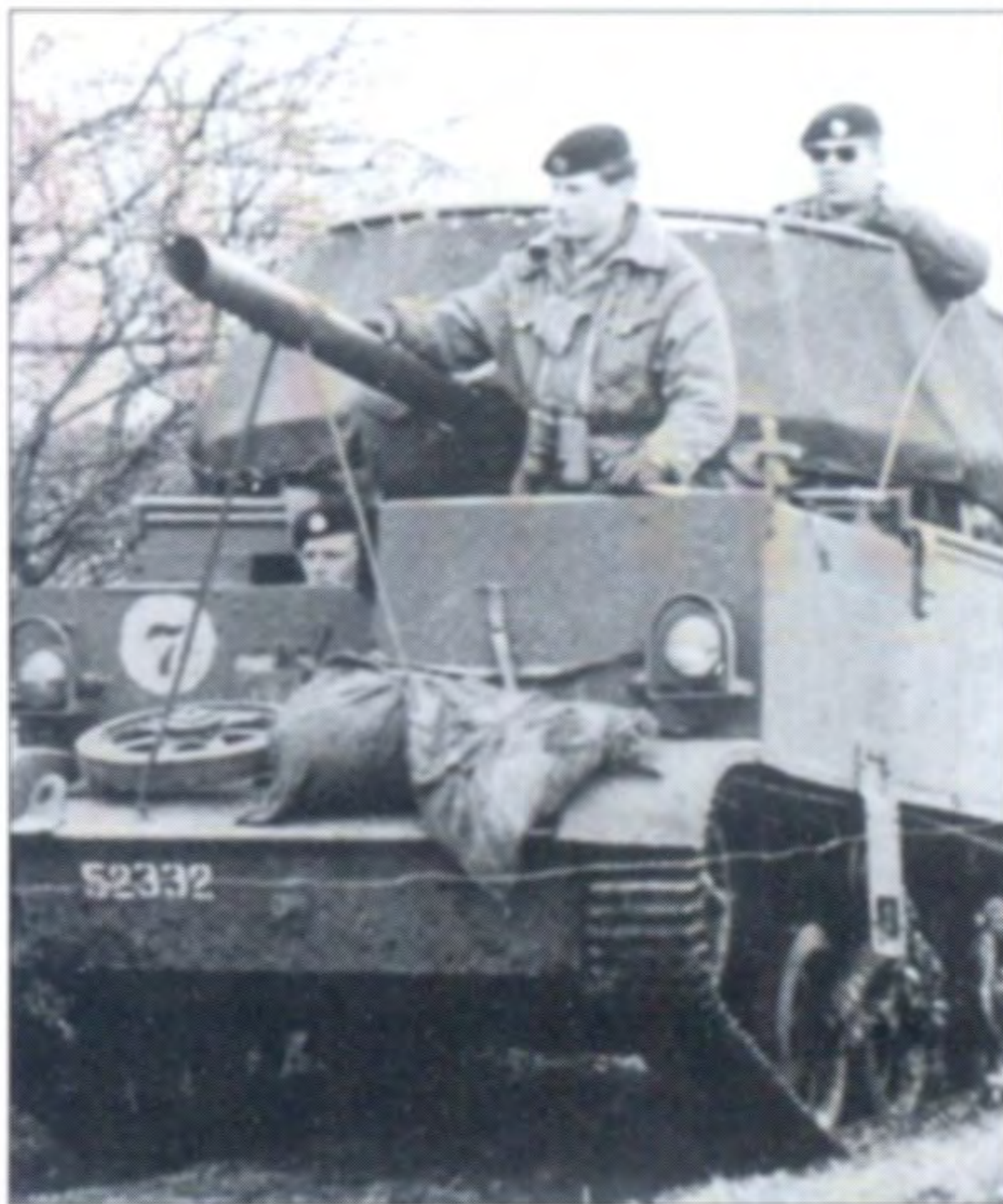
Danish troops with an extensively modified Mark II Universal. The weapon could be a 106mm recoilless anti-tank gun or simply a length of tube which, in conjunction with the canvas screen, might be intended to represent a turreted tank for training purposes.
