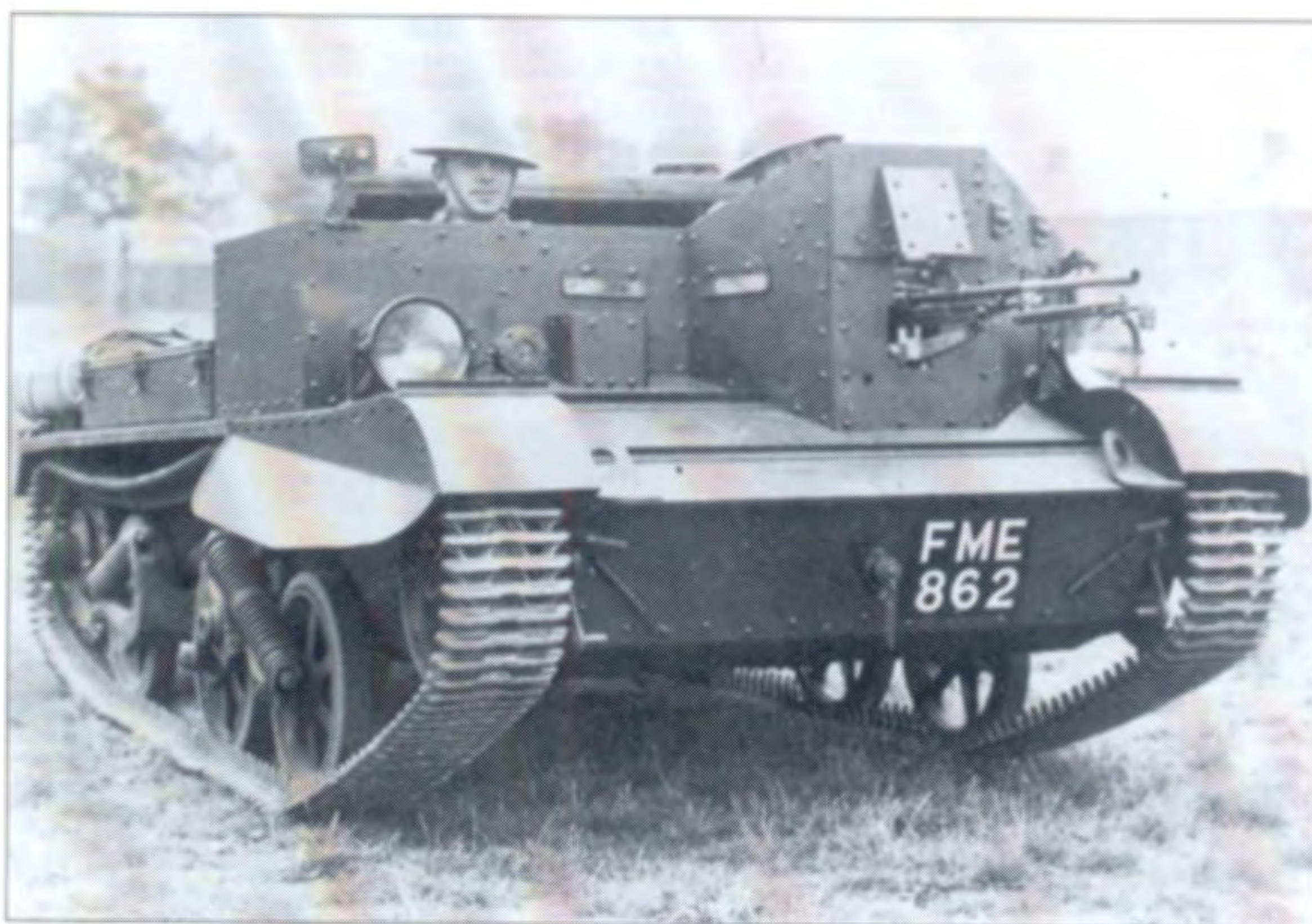
A Bren Carrier that started life as a Machine Gun Carrier No. 2 Mark I. The support for the Bren gun shows up well as do the protected visors for the driver and gunner. The plug in the nose plate, just inboard of the registration number, covers the hole for the engine starting handle.
