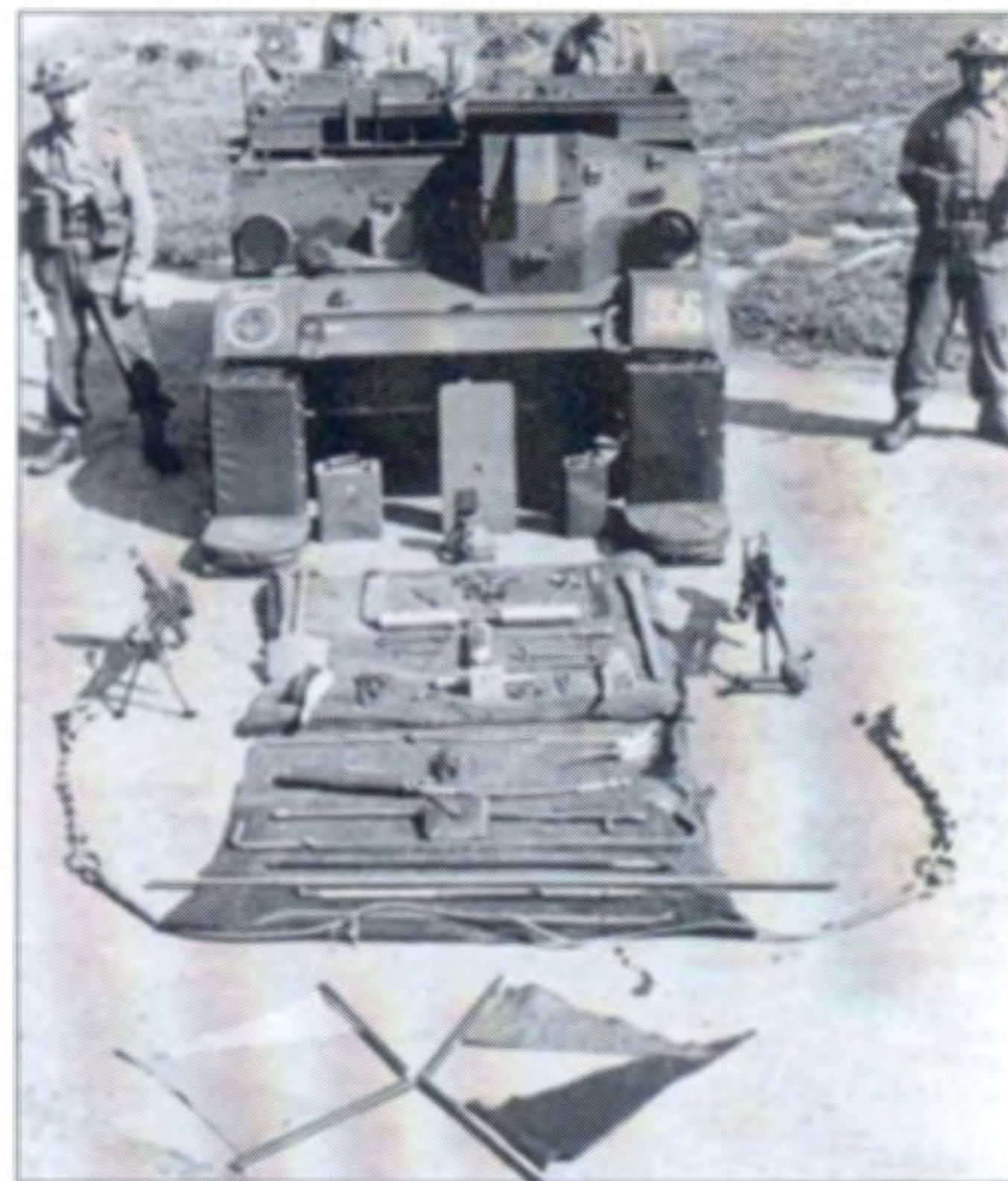
A Universal Carrier Mark I with everything laid out for inspection and crew members in place. In a small vehicle such as this, efficiency requires that these items are stowed to plan so that everyone knows where they are. To this end the War Office produced a series of special stowage diagrams, which, in the case of carriers, cover most primary roles. Note in particular the Bren gun, Boys rifle and signal flags.
