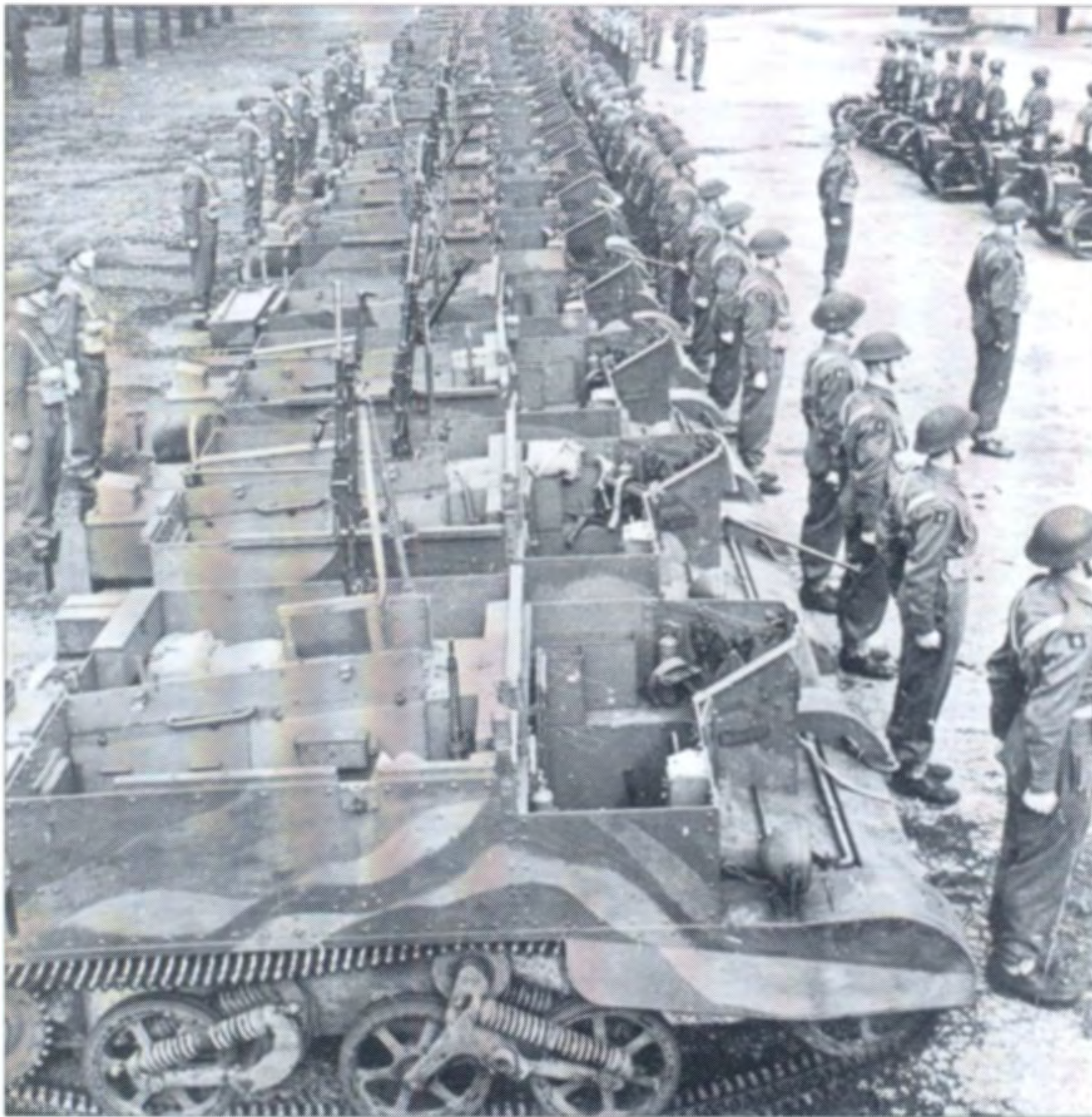
Mark I Universals of the Scots Guards in a most unusual camouflage scheme. There are more vehicles here than one would expect to find in the carrier platoon of a rifle battalion but the presence of Norton 633 motorcycle sidecar units suggests an early date. Some carriers mount a Boys rifle at the front while all appear to have the pillar-mounted Bren gun and a few the 2in mortar.
