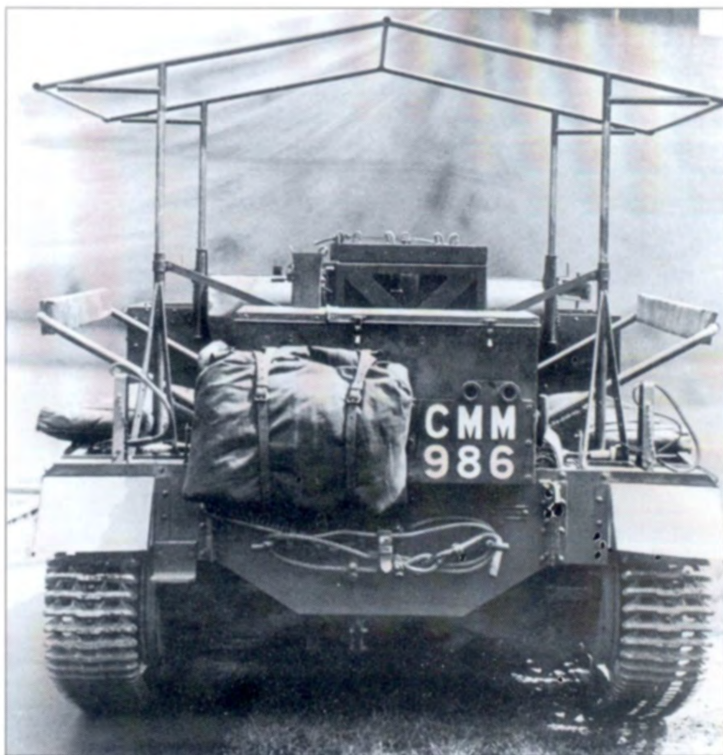
The prototype Cavalry Carrier photographed from the rear. Padded squabs and backrest for the rear passengers can be seen along with the frame for its canvas hood. There is a large locker at the back and two more above the engine, one of which has clips for the men's rifles.
