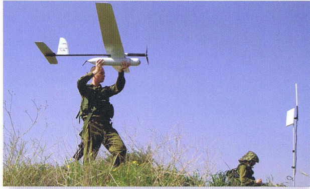
Elbit's Skylark IV was used by the Israeli Defense Force for patrols over Gaza and Lebanon during the turmoil in 2006. This design uses an electric engine and so is virtually silent in flight. (Elbit)
