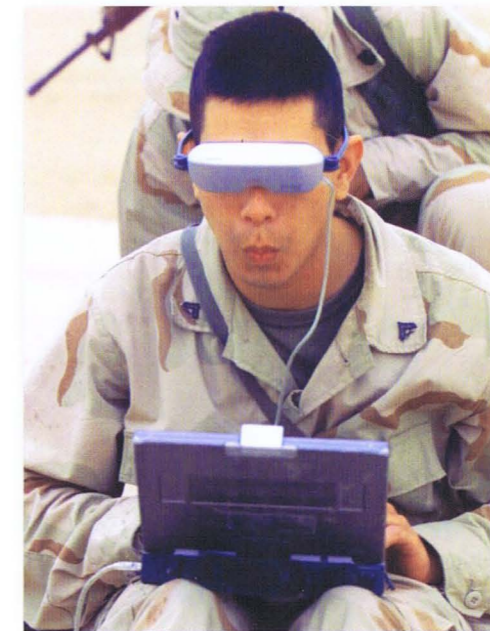
The advent of miniaturized computer processors permits mini-UAVs to be operated by laptop computers. This Marine from the 3rd Light Armored Reconnaissance Battalion is flying a Dragon Eye mini-UAV on a scouting mission from Camp Ripper, Kuwait, in March 2003 using special semitransparent eyeglasses that display moving map imagery of the mission while other imagery is provided by the laptop screen on his knees. (US Marine Corps)
