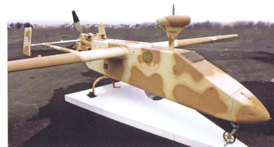
Israeli Aircraft Division's Malat division was one of the pioneers of the new generation of tactical UAVs that could provide real-time intelligence using commercial video cameras. The Searcher was a further evolution of the Scout, which was used in the 1982 Lebanon war, and proved to be one of the most widely exported UAVs of the 1990s. (Author)
