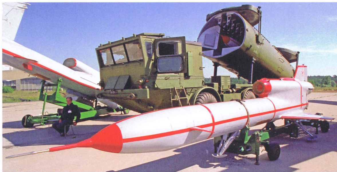
The most widely used Soviet spy drone of the Cold War was the VR-3 Reys based on the Tu-143. This shows the improved VR-3D Reys-D with the Tu-243 drone and the SPU-243 launch vehicle behind. (Author)
