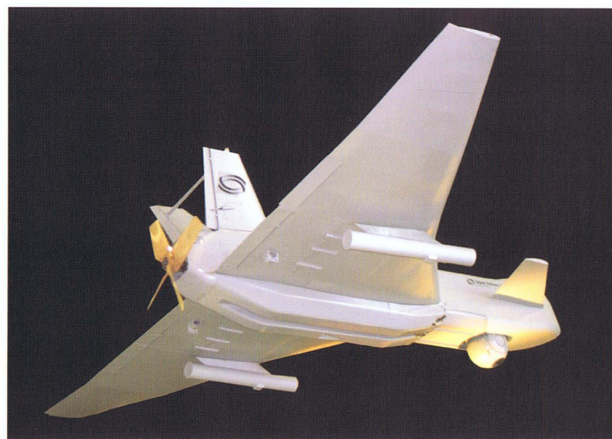
France has been exploring hunter-killer UAVs with an armed version of its popular Sperwer tactical UAV, seen here in the armed Sperwer B configuration with missile launchers under the wing. (Author)
