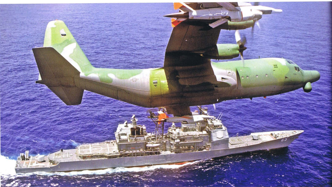
The DC-130 served as the mother ship for Firebee drones during the Vietnam War. This DC-130 is in use by the US Air Force's 6514th Test Squadron, hosting AQM-34 Firebee target drones to test air defense systems like those on Aegis cruiser USS Chosin seen below in May 1991. (US Navy)
