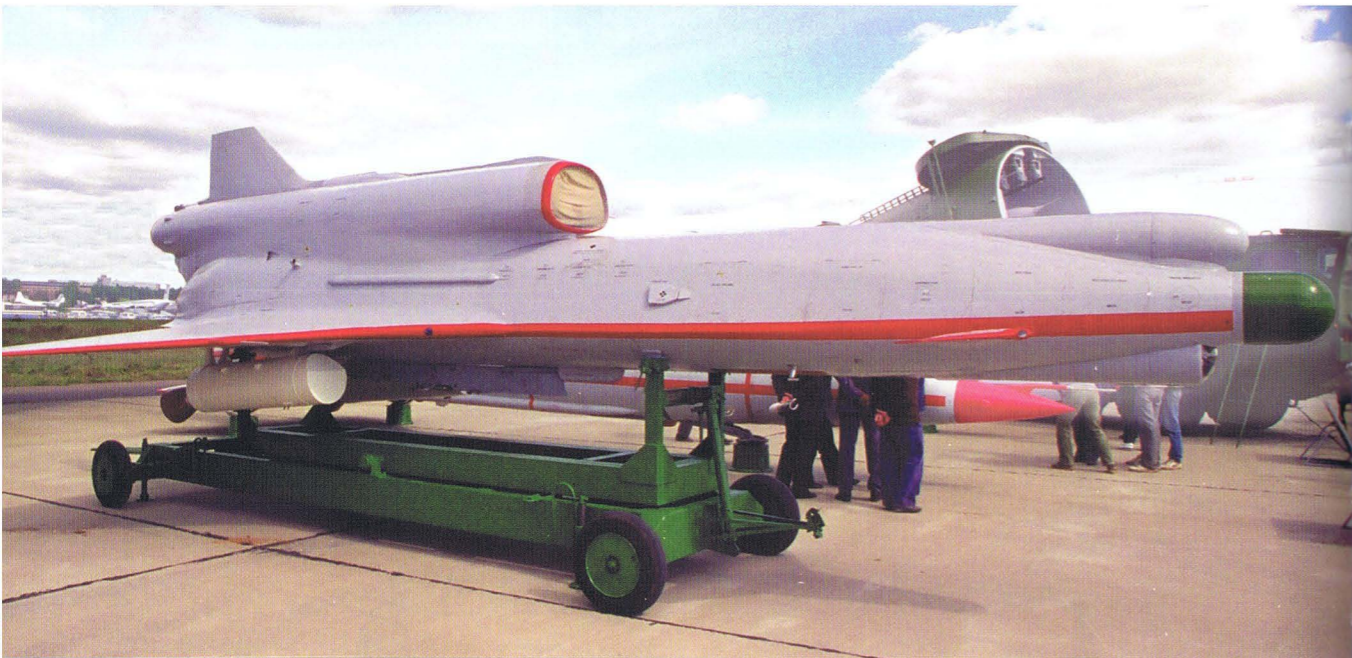
Russia's assault drone program has remained shrouded in mystery, although this Tupolev Tu-300 Korshun was displayed at the Moscow Air Show in 1995. It carries its weapons in an internal bomb bay or on an external pylon and has sensors on the nose for remote piloting and target detection. (Author)
