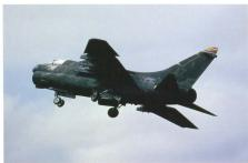
Above Not all Arizona Air Guard A-7s wear the attractive grey colours, this example being one of a small minority still sprayed in the now unfashionable 1980s charcoal scheme. Being matt-based, the paint applied to the A-7s was very porous and tended to absorb moisture, thus resulting in greater corrosion problems for the groundcrews and the aircraft looking generally scruft.
