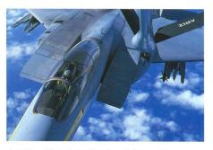
Above 'Mongo' Sakai holds his jet in position as the IP4 is carefully pumped from the internal tanks of the KC-135E into his F-15. The sniper scope mentioned earlier is clearly visible mounted on the instrument coaming to the left of the HUD. Reflecting in the Eagle's crystal clear canopy is the traffic light-coloured refuelling boom, painted not for the boomer's amusement but to help the receiver judge his separation distances from the tanker
