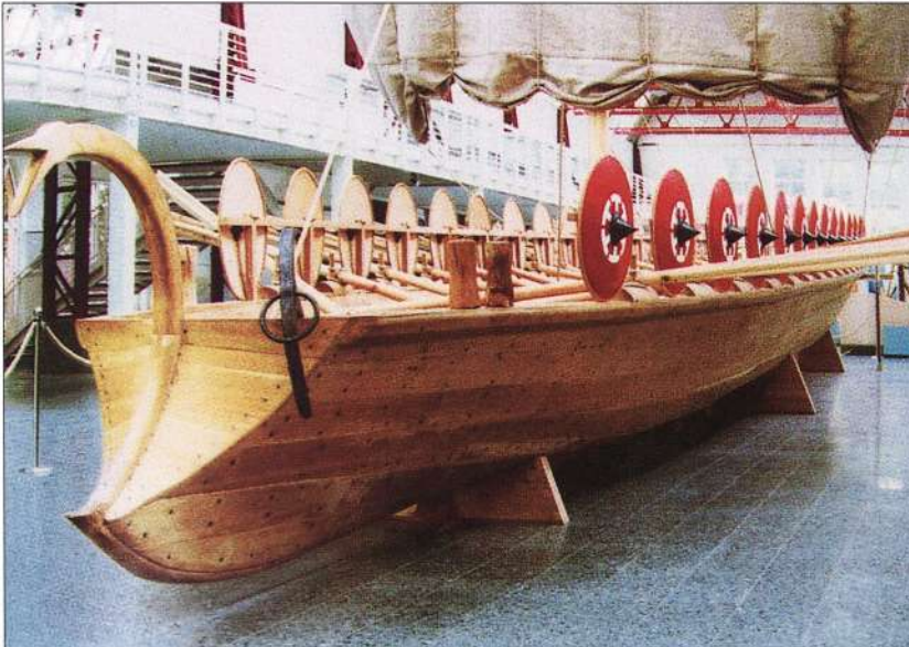
Reconstruction (Mainz, Museum für Antike Seefahrt) of one of the 4th-century wrecked craft from the middle Rhine. The original (Mainz A) was a wide, flat-bottomed vessel with near vertical sides. It has been identified as a light warship some 21m long and with an oarcrew of 30. (Esther Carré)
