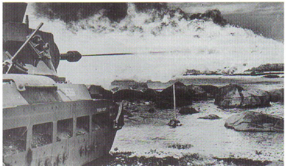
A Matilda Frog flamethrower blazing away at maximum range with considerable effect. Despite what was, in fact, a fairly complicated conversion the tank appears to be almost unaltered from the outside. (The Tank Museum, Bovington)
