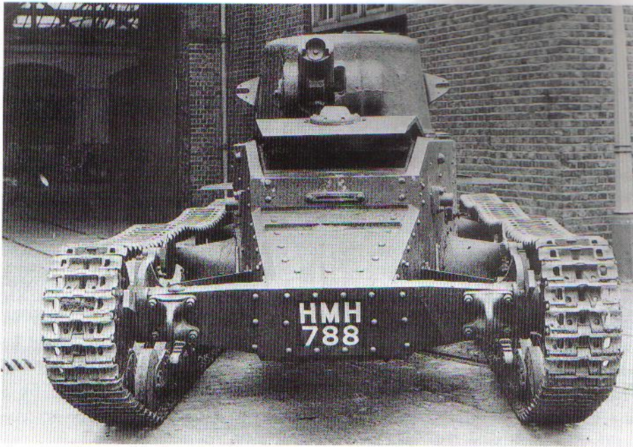
HMH788 (T3433) was the first production A11. This front view shows the new arrangement of the front hull plate and the typical Vickers track adjusting mechanism. Other features to observe are the driver's narrow vision slit and periscope, in his hatch. On the turret one can see two mountings for the smoke dischargers and notice the lack of the prominent lip seen on the prototype. (Vickers-Armstrongs)
