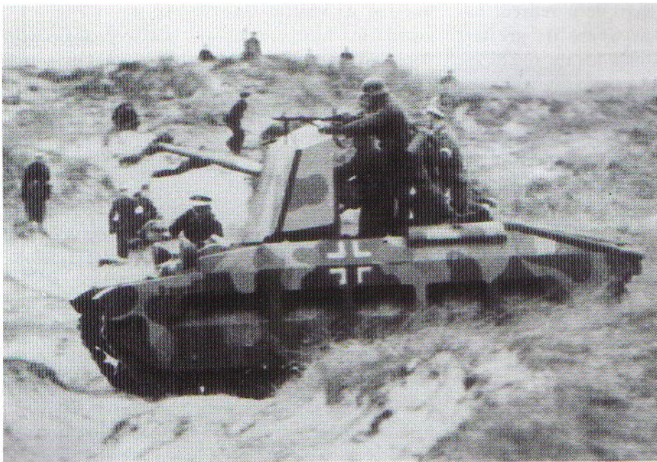
In German hands the Matilda was known as the Infanterie Panzer Mk II 748(e). This is the example nicknamed Oswald converted to mount the 50mm tank gun, seen here on a training exercise at Terneuzen. (The Tank Museum, Bovington)
