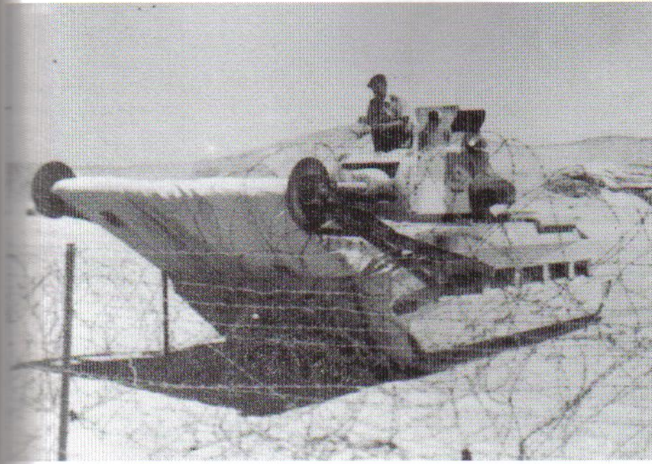
The original carpet device on a Matilda being demonstrated on a barbed wire entanglement. (The Tank Museum, Bovington)
