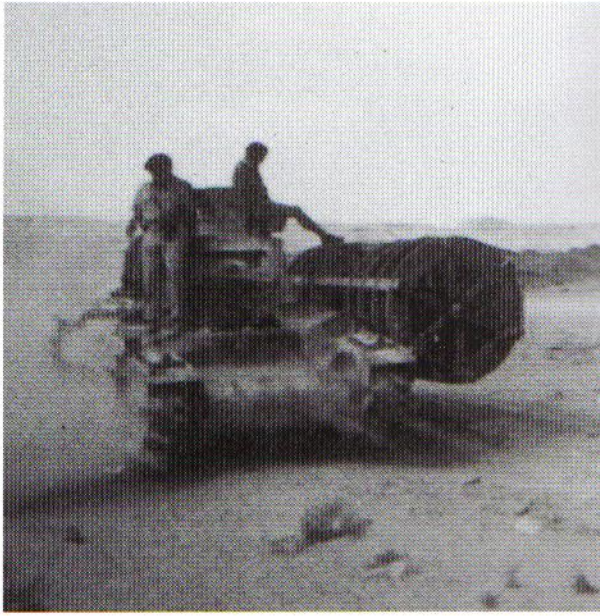
A poor but interesting picture of a 7th RTR Matilda carrying a large fascine during trials at Halfaya. Notice that to save weight, and
