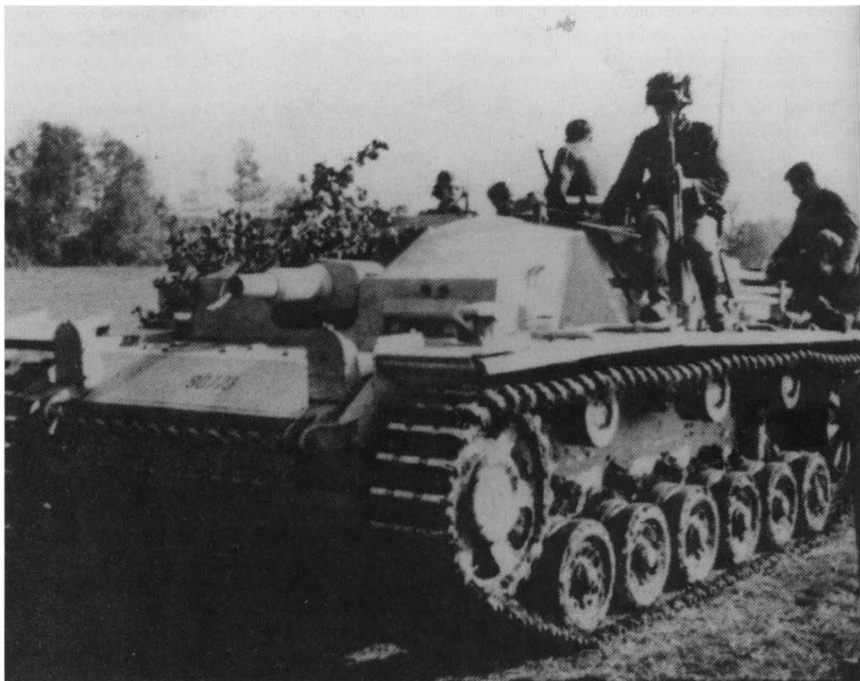
A Sturmgeschütz Ausf. E (Fgst. Nr. 90773) with the superstructure of an Ausf. D – an arrangement which typifies the gradual changes introduced to the vehicle during its production run.
