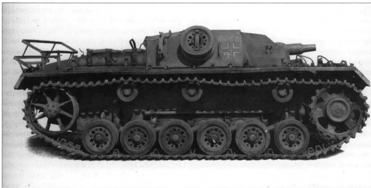
Sturmgeschütz Ausf.D (Fgst.Nr. 90683) was one of three Sturmgeschütz which served in North Africa with Sonder Verband 288. This was a tropicalised vehicle with addi-
