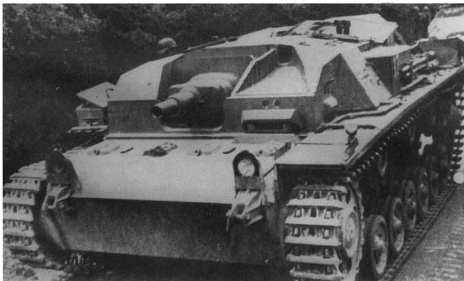
One of the Sturmgeschütz Ausf. A of 16 SturmBatterie/ Infanterie-Regiment 'Gross-Deutschland' during the campaign in France 1940. This unit took delivery of the first six Ausf. A's. Note the mixture of narrow and wide wheels.
