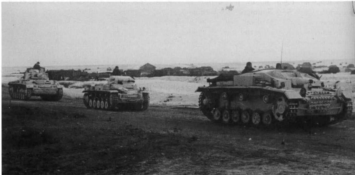
Sturmgeschütz Ausf. E of Sturmgeschütz-Abteilung 192 overpainted in whitewash for the Russian winter. (Author)
