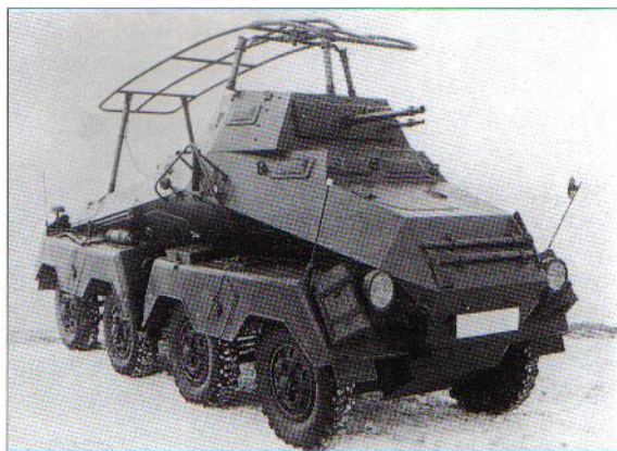
SdKfz 232 Schwere Panzerspähwagen (8-rad) (Fu) in mint condition. The photo clearly illustrates the working of the swivel aerial mounting which permitted the turret all-round traverse. (Bundesarchiv)
