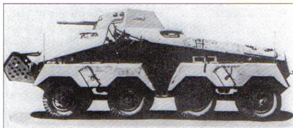
SdKfz 231 (8-rad) with barrier shield. The front and rear driving positions can be identified by the visors in the hull side. (RAC Tank Museum)
