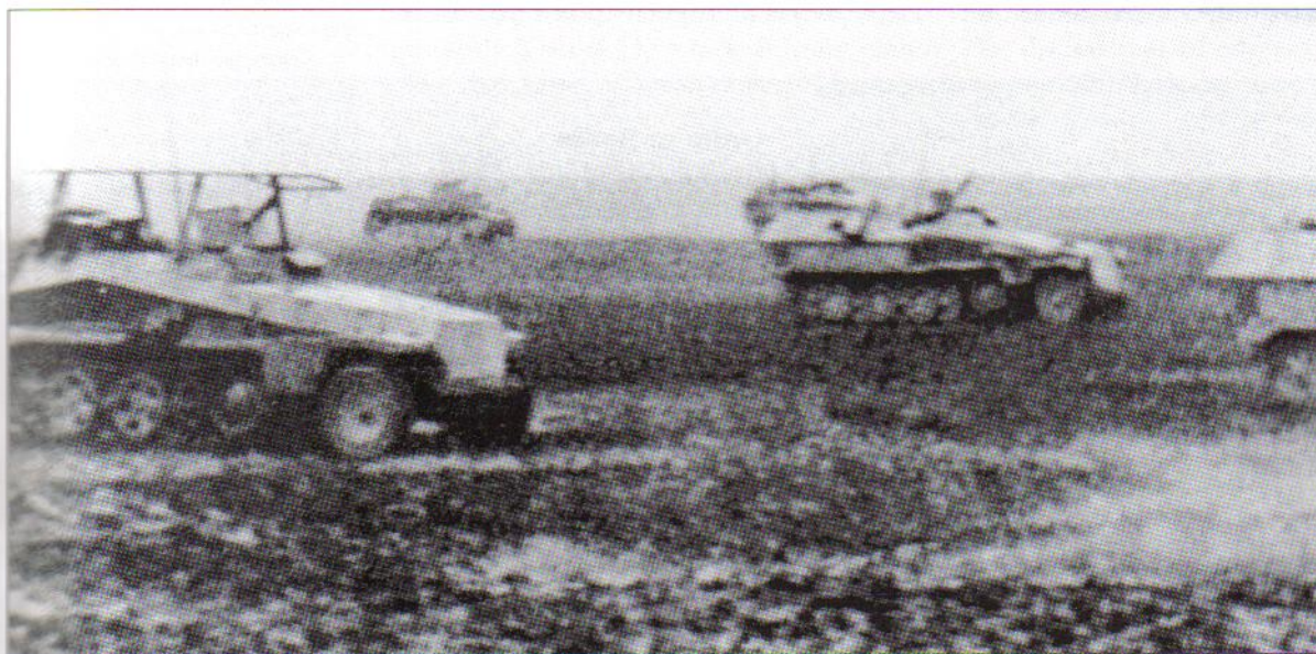
An SdKfz 250/3 command vehicle on the move with a Panzergrenadier battlegroup including several of its larger SdKfz 251 cousins and a PzKpfw II. Russia, 1942. (US National Archives)
