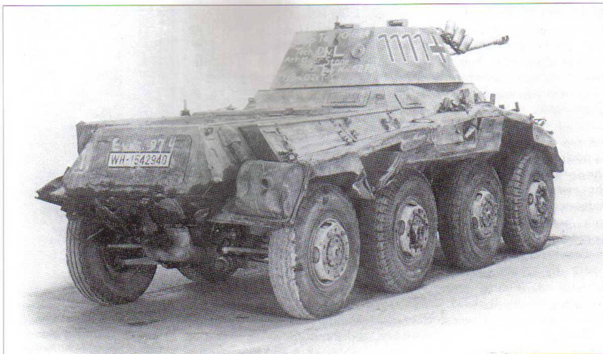
Three-quarter rear view of a Puma captured in badly battered condition. The colour scheme is standard ochre with an oversprayed mottle of green and brown. The use of such prominent black and white turret numbers and national crosses is quite at variance with normal armoured car practice, since they were hardly an aid to concealment. The rear turret markings indicate that the vehicle is on the point of being back-loaded for evaluation by Allied ordnance. (RAC Tank Museum)
