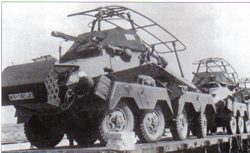
Clearly-marked SdKfz 232 (8-rad) (Fu) of the 1st Armoured Reconnaissance Sqn., Panzer-Aufklärungs-Abteilung 'Grossdeutschland' in rail transit near Kursk, June 1942. The turrets have been sheeted down, and each bears the Reichsbahn's shipping label. The leading car has been fitted with a frontal shield with which to force its way through barriers. The slight right-hand lock illustrates perfectly the effect of eight-wheel steering. (Bundesarchiv)
