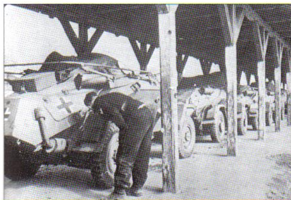
Light armoured cars awaiting rail transport to the front, summer 1942, protected by the rail-head's permanent overhead canopies from enemy aerial observation. Closest to the camera are two SdKfz 223s with an SdKfz 261 Kleiner Panzerfunkwagen between them; further down the line are several SdKfz 222s. (Martin Windrow)
