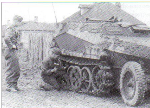
SdKfz 250/1 with suspension problems: Russia, autumn 1941. The use of hammer and cold chisel seems to imply stones jammed between the bogies, a common complaint of interleaved suspensions. The long bonnet of the 250 series gave a large reflective area, which this crew have countered by applying a thick coat of mud. The left-hand man wears what seems to be the assault artillery uniform; later in the war some recon units seem to have adopted it, with suitable changes of insignia. (Bundesarchiv)
