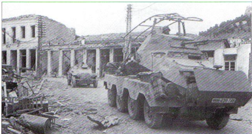
An SdKfz 232 (8-rad) (Fu) leads the way through a ruined Greek village, spring 1941. Some attempt seems to have been made to overpaint the original 'Panzer grey' scheme with a light (sand?) shade, but much of this has worn off, and the barrier shield has not been repainted at all. The name 'Seydlitz' appears on the hull side in white Gothic script. The second vehicle is an SdKfz 221 light armoured car, mounting a smaller turret than the 222. (Bundesarchiv)
