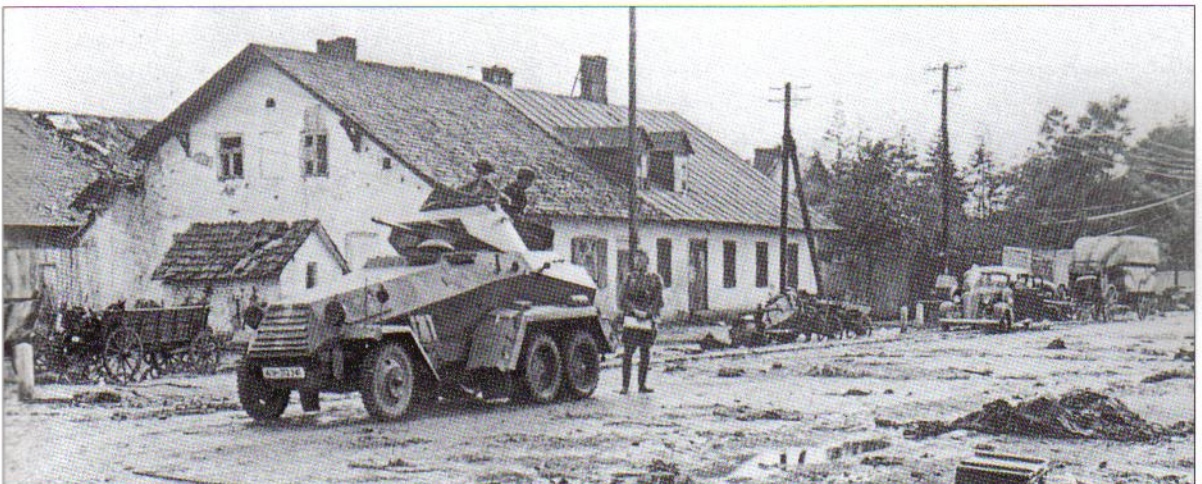
SdKfz 231 (6-rad) heavy armoured car in a battle-damaged village in Poland, September 1939. The large national cross on the radiator louvres, originally white, seems to have been overpainted yellow; another cross on the hull side has been completely masked. Ahead of it is a yellow W, significance unknown. (Bundesarchiv)
