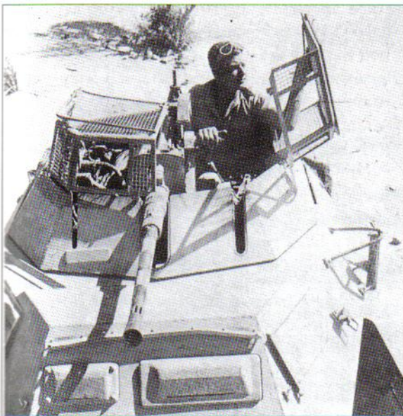
Detail of the 20mm mounting and anti-grenade grilles of an SdKfz 222 – the co-axial MG is absent. (RAC Tank Museum)
