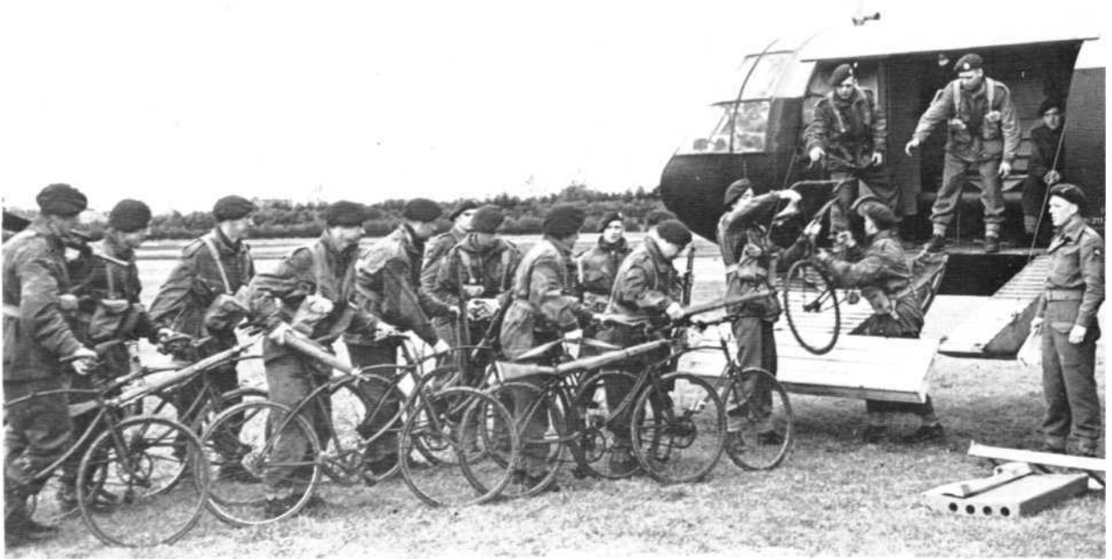
Loading a Horsa Mk. 1 glider; the wide door behind the cockpit was designed to take a jeep, and there were two smaller doors for personnel at the rear of the fuselage. These Royal Engineers (?) are loading the famous 'Airborne Bicycle', a folding machine used mainly by communications troops; some men jumped with them, others were dropped under their own 'chutes, (ABF Museum)
