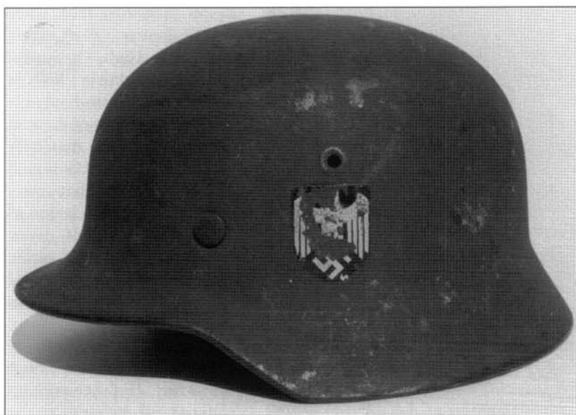
This M1940 helmet displays a non-reflective textured finish common to helmets delivered after 21 March 1940. The decal insignia has chipped off as a result of the rough painted surface.
