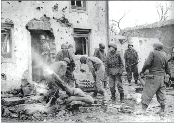
Baal, Germany, February 1945: a 4.2in heavy mortar of a US Chemical Mortar Battalion, caught at the moment of discharge at a shallow angle, while supporting the infantry clearing the town. Boards and a heap of sandbags are used to prevent the heavy recoil from moving the weapon or driving the baseplate into the soft ground. Although originally intended primarily for the delivery of smoke – thus the designation of the units equipped with it – the 4.2in packed a heavy high-trajectory punch that was useful in built-up areas. (US Signal Corps)
