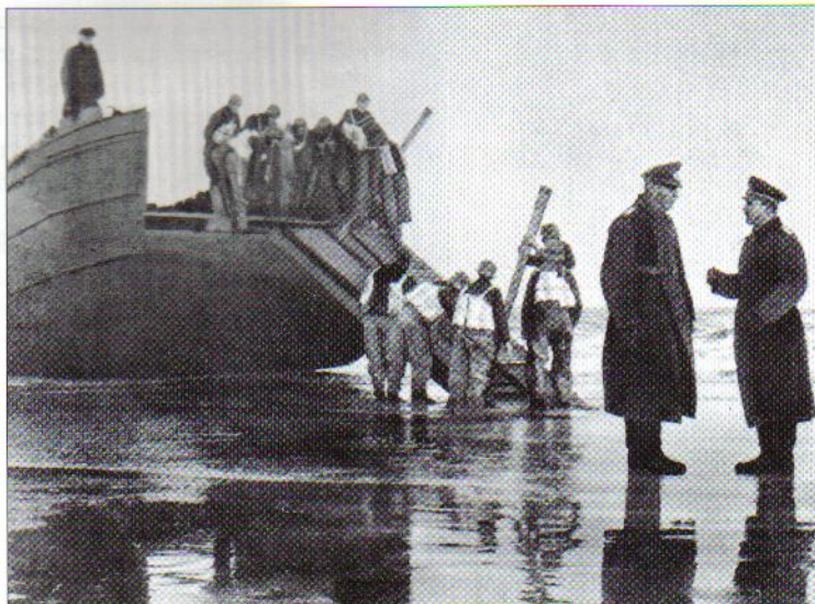
German sailors practice disembarking from a converted barge: the bows have been removed, a false floor fitted and stakes are being positioned to secure the ramp. In the foreground Heer officers confer. (IWM HU 2790)
