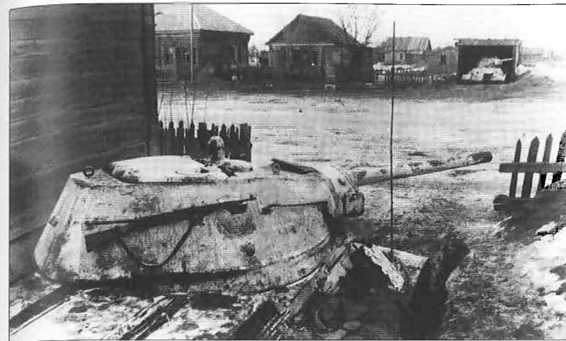
A T-34/76 tank is emplaced in a hull-defilade pit, which would enable it to fire. Across the road another tank is partly dug in under a shed. The tanks have been winter whitewashed. Note the German 7.9mm Kar.98k carbine in a handy position to take potshots at targets of opportunity. (CMAF)
