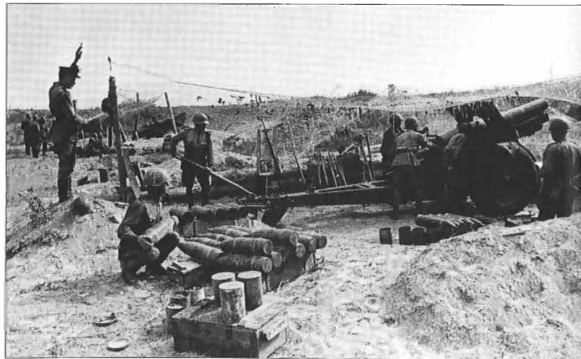
A 152mm M-1910/30 howitzer, mainly assigned to second-line formations, is emplaced in a typical artillery position. The camouflage net does little to conceal the exposed parapet and equipment around the position, but does deny observers from determining the type of weapon. (RGAKFD)
