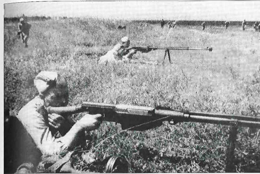
Anti-tank rifle crews are shown here taking up hasty positions. They are armed with the semi-automatic 14.5mm PTRS-41. The shear bulk and size of these weapons can be appreciated in this photograph. The assistant gunners are armed with 7.62mm PPSH-41 submachine guns, but could be armed with rifles. (Author's collection)
