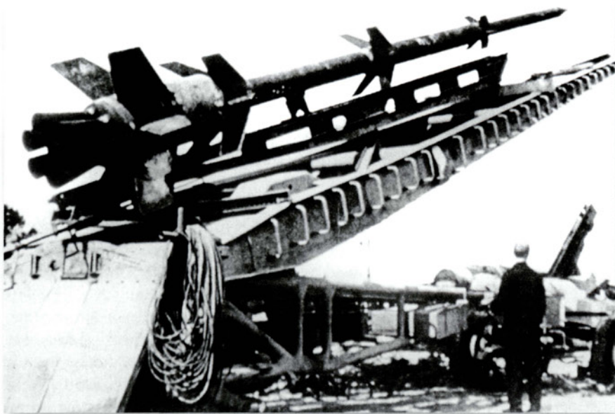
The Rheinbote rocket was launched from a simple rail mounted on a V-2 Meillerwagen transporter-erector fitted with a blast deflector at the rear. As a result it had no precise traverse, degrading the already poor accuracy of the weapon. (NARA)
