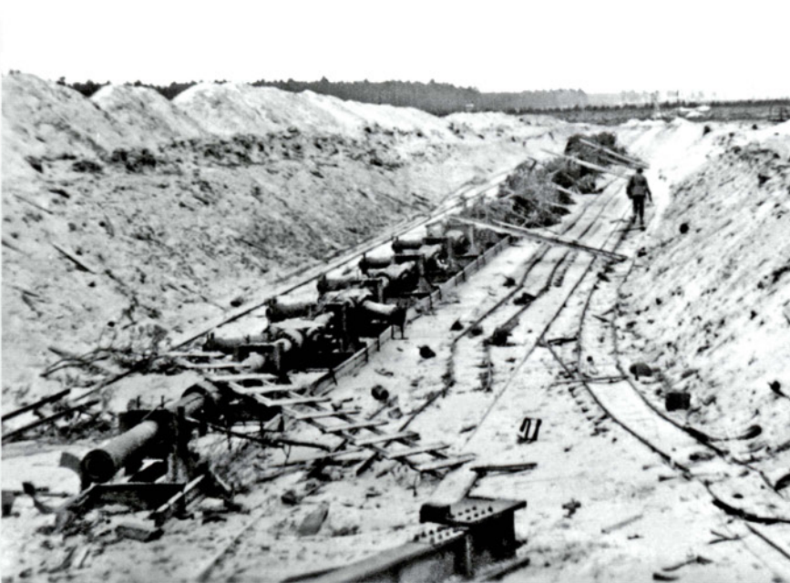
This shows a test version of the Tausenfüßler HDP supergun at the Wehrmacht's Hillersleben artillery test range after its capture in 1945. (MHI)
