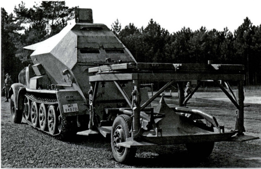
The Meiller launch pad was towed to the launch site, in this case behind the SdKfz 7 8-ton half-track armored fire-control vehicle. The wheeled trailer was removed before the missile was placed on the pad. (NARA)
