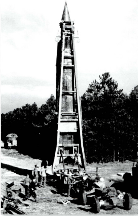
The V-2 launch site was generally created in wooded areas to help camouflage the launcher, but an extensive road network was needed for the many support vehicles. (NARA)
