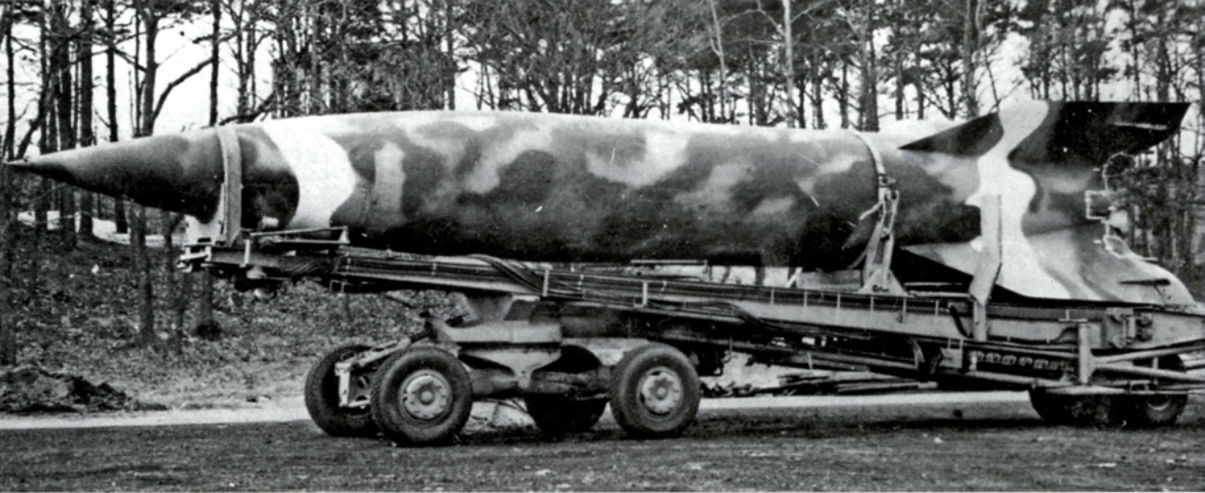
In the mobile batteries, the A-4 missile was towed to the launch site on a Meillerwagen, which erected the missile on the launch pad prior to fueling. (MHI)
