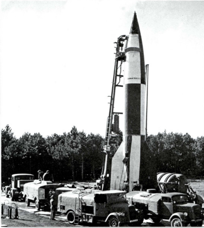
After the missile was erected on the launch pad, the V-2 service battery deployed a variety of fuel trucks, pump trailers and other support equipment to fuel the missile, as seen in this test launch conducted for the Allies in 1946. (NARA)
