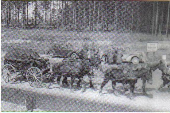
Hf1 waggon, here with a camouflage-painted canvas cover, and a four-horse hitch rather than the usual pair. The larger Hf2, which always needed a four-horse team when in the field, was used by supply columns but was too unwieldy for a cavalry squadron transport. So was the steel-bodied Hf7/11 with rubber-tired wheels, which was issued in quantity to horsed units shortly before the war; with an empty weight of 1,040kg (2,292lbs – just over a ton), it had a load capacity of 1,720kg (3,792lbs – another 1.7 tons). (Paul L.Johnson Collection)
