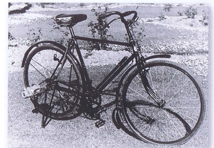
A bicycle has been fitted with a pedal generator to charge the batteries of a wireless set. (IWM HU56739)
