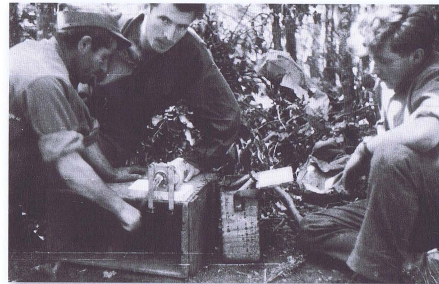
Partisans charging a radio battery with a hand-operated dynamo, Macedonia, July 1944. (IWM HU67330)
