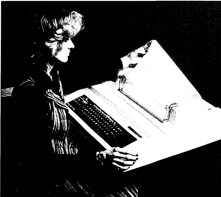
Fig. 1.7 A printing terminal ( © Digital Equipment Corp. All rights reserved. Reprinted with permission.)
