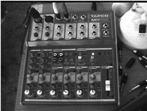
FIGURE 6.3 A ten-channel audio mixer.
