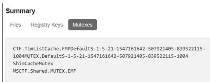
Figure 3-8: The Mutexes tab of the Summary pane, showing which mutexes our malware sample created
