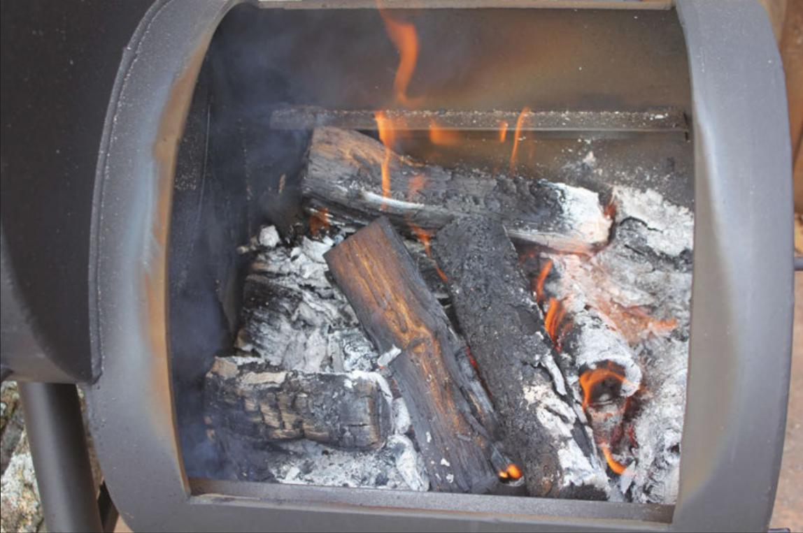
**ABOVE:** The big firebox on the Horizon, separate from the meat-cooking area, provides plenty of space for loading lots of fuel for long cooking times.
