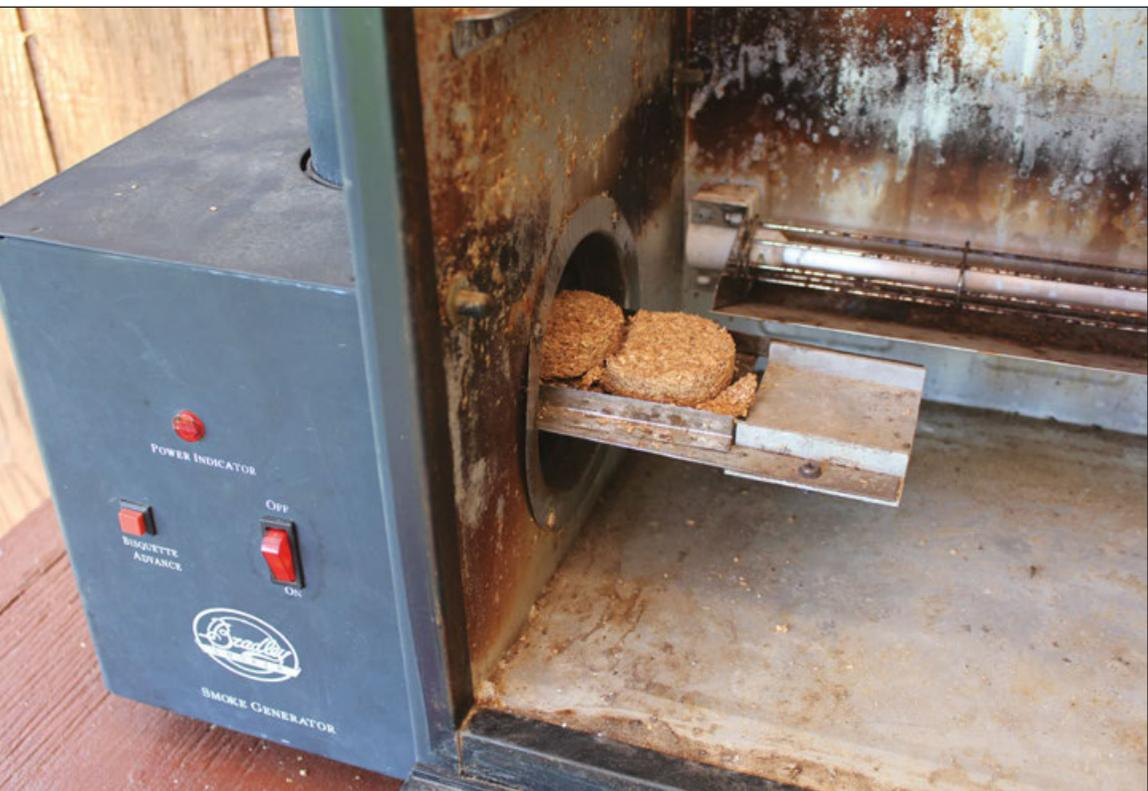
**ABOVE:** The smoke generator feeds bisquettes at a precise burn time of 20 minutes per bisquette.
